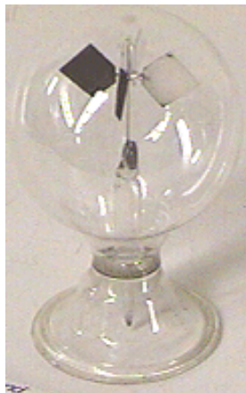
Fig. 1.7 A Crooke's Radiometer enclosed in an evacuated bulb. Light creates a thermal gradient across the vane. The effects of thermal creep then create a pressure difference which in turn, moves the vane away from the hot gas.
