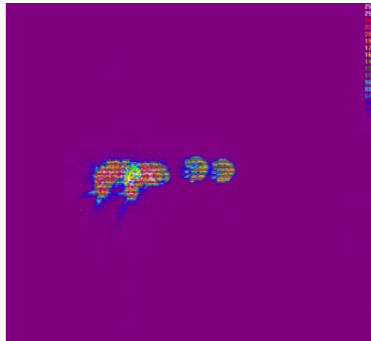
Figure 3.5 & 3.6 Charcoal particle(s) in a 4.5 watt laser beam. Figure 3.5 shows the particle moving 15 \mu in 1/60 seconds with an average speed of 0.9 \times 10^{-3} m/s. Several minutes later the original particle becomes coupled with a 10 \mu size particle as seen in Figure 3.12. 125x117 \mu window size
