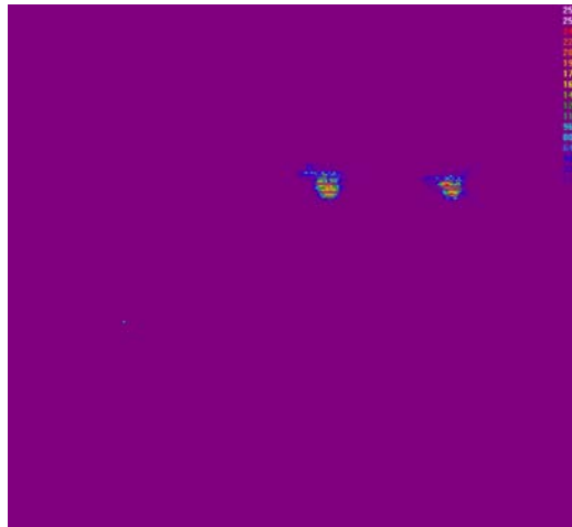
Figure 3.1 6 \mu size Tungsten particle in 4.5 Watt laser beam The particle moves 27 \mu in 1/60 seconds with an average speed of 1.6 \times 10^{-3} m/s, 125x117 \mu window
