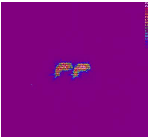
Figure 3.5 & 3.6 Charcoal particle(s) in a 4.5 watt laser beam. Figure 3.5 shows the particle moving 15 \mu in 1/60 seconds with an average speed of 0.9 \times 10^{-3} m/s. Several minutes later the original particle becomes coupled with a 10 \mu size particle as seen in Figure 3.12. 125x117 \mu window size
