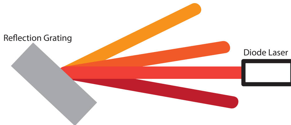
Figure 1.1 In an extended-cavity diode laser a reflection grating reflects a specific frequency of light back into the laser diode. Here the frequencies are illustrated by different colors.
