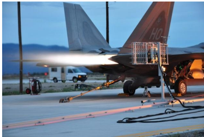
Figure 30: F-22 Raptor tethered to the run-up pad. The 90-microphone array is shown on the track that allowed it to move in 2.3 m increments horizontally, parallel to the shear layer, and 0.6 m increments vertically.
