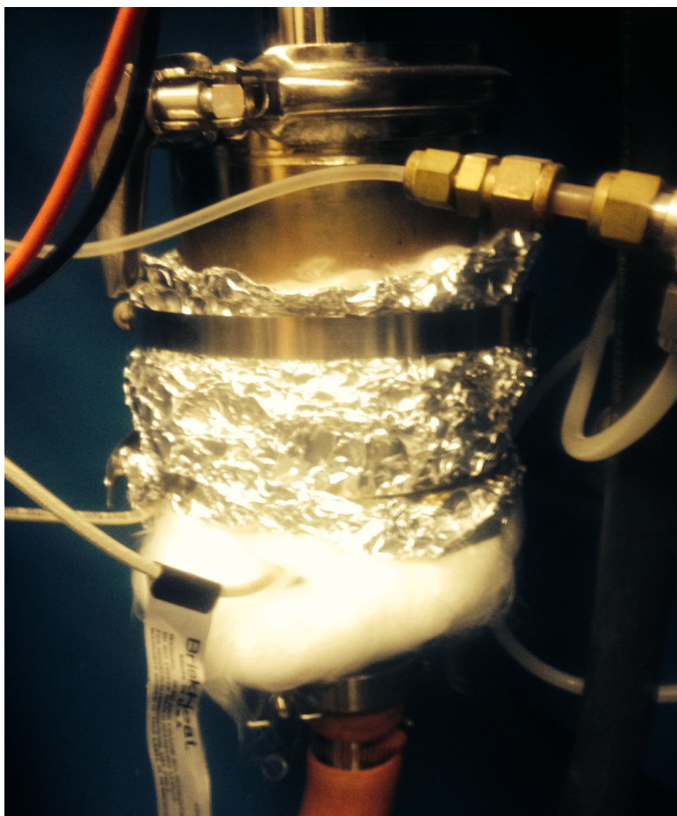
Figure 2.5 A picture of the HF trap we placed between the sample chamber and roughing pump. This was filled with steel wool and aluminum shavings to help diffuse the HF gas before it reached the pump.
