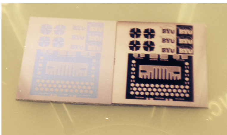
Figure 2.1 Two segments of a silicon wafer side by side. The sample on the left has gone through lithography and iron deposition. The sample on the right has carbon nanotubes grown on it.
