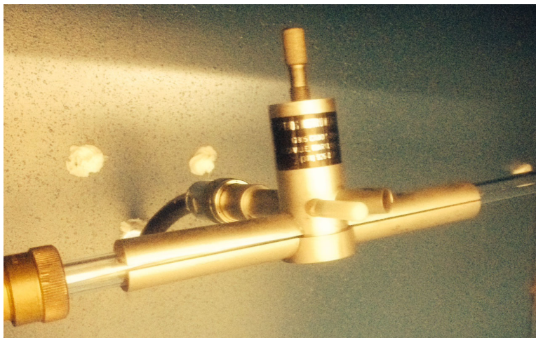
Figure 2.3 The antenna for the microwave generator clamped around a quartz tube.
