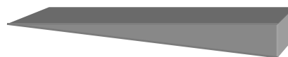
Figure 5: Example of a wedge sample. The tip is polished to be electron transparent (<100 nm).
