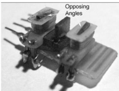
*Figure 1:* Freed and Isvan's designed multi-axes guitar pickup.
