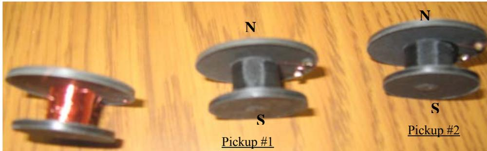
Figure 5: Uncovered magnetic pickup, magnetic polarity of Pickup's #1 and #2.
