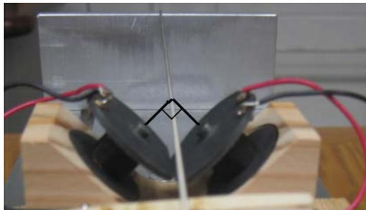
*Figure 2:* The two-dimensional guitar pickup designed for the experiment.
