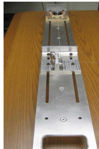
*Figure 4:* The final manufactured monochord.
