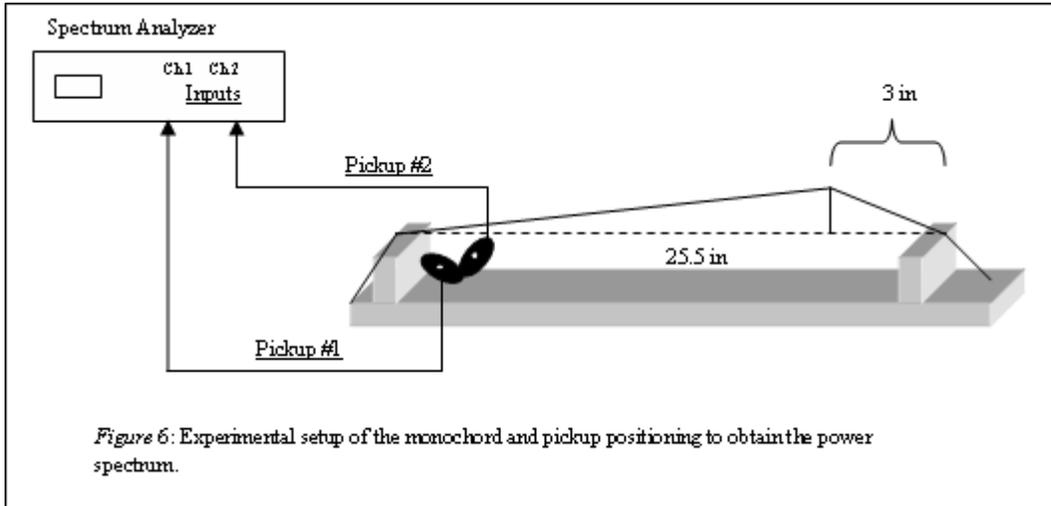
For the actual process of retrieving the frequency response of the system, a broadband random signal of 5 peak volts was sent through the output of the analyzer to a Ling Dynamic System shaker and to the input of Channel 1. Pickup #1 and pickup #2 were connected to the inputs of Channel 2 and Channel 3 respectively.
