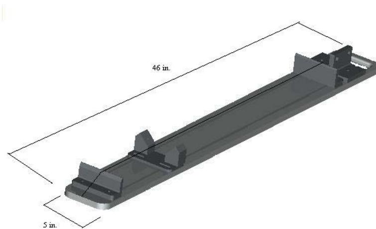
*Figure 3:* The SolidWorks monochord design for the experiment.
