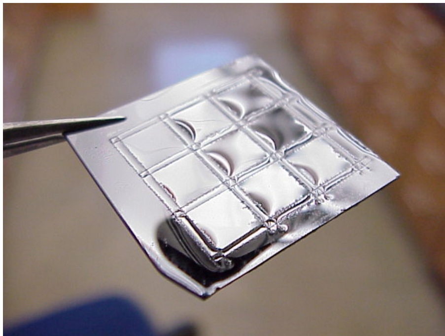
Figure 2: Hydrophilic patches surrounded by a hydrophobic matrix of lines after a rinse with DI water.
