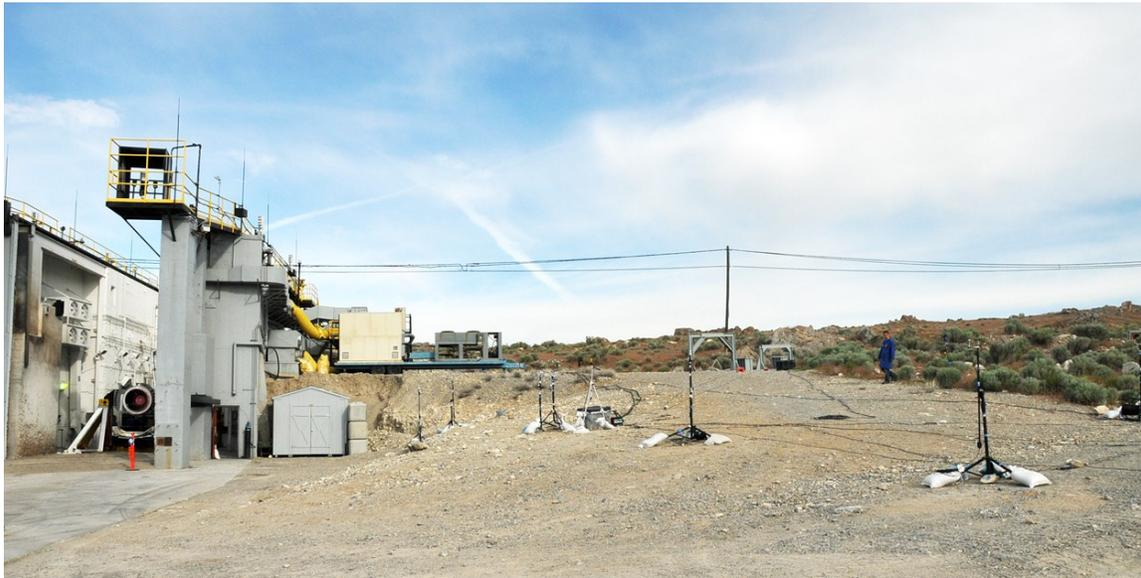
**Figure 2.4** The microphone layout that was used in the Orion 50 test and its general orientation to the rocket.
