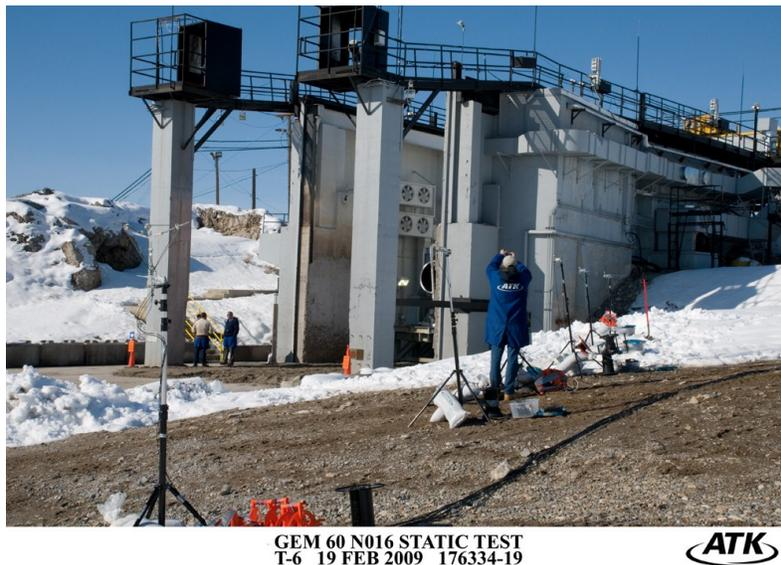
Figure 2.6 The microphone layout that was used for the GEM 60 test and its general orientation to the rocket.
