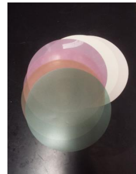
Figure 4: Diamond lapping films green (30 \mu\text{m} ) down to white (0.1 \mu\text{m} )
