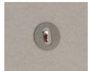
Figure 7: Finished polished sample on grid. Width of grid = 3mm
