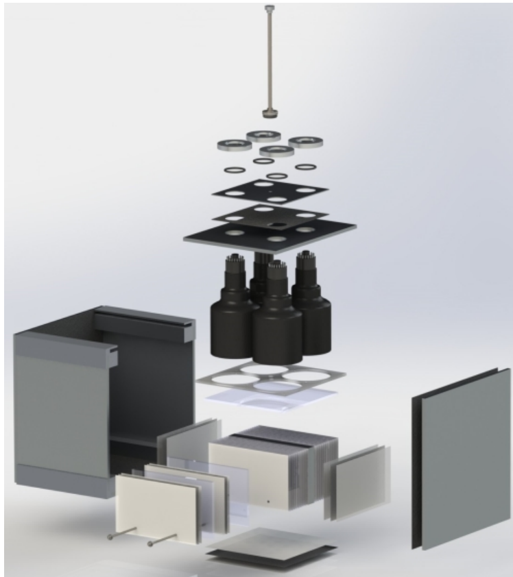
Figure 1.4 An exploded diagram of the 4-fold detector
