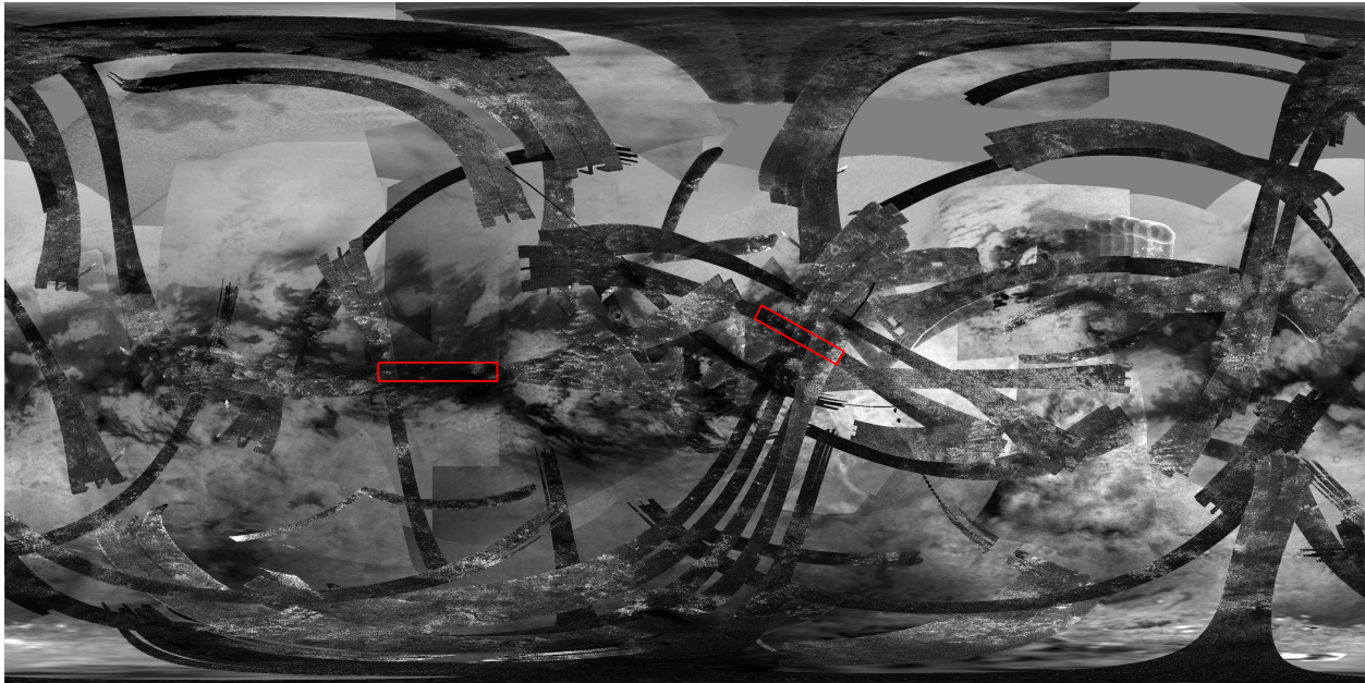
Figure 2.2 A map of the surface of Titan. The base map was taken using the Cassini ISS instrument. Radar swaths are overlaid on the base map. The red box on the left is the T08 swath, and the red box on the right is from the T44 swath.
