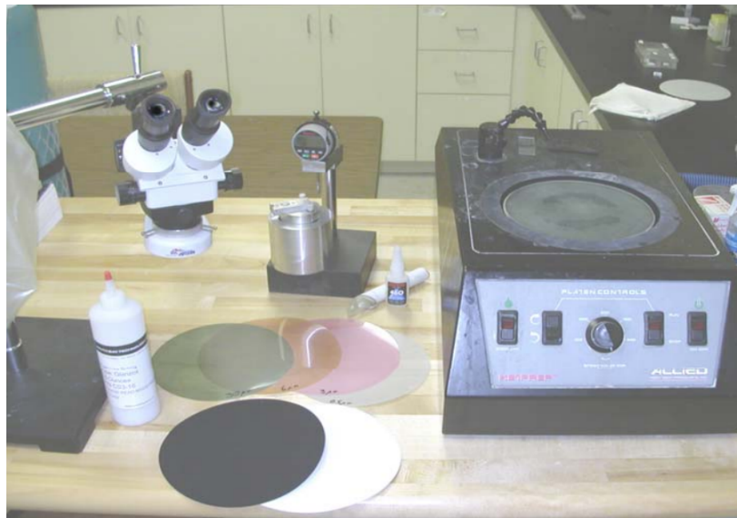
Figure 6: Tripod polishing setup, with the polisher on the right and the micrometer in the center. Note the multiple diamond lapping films: 30 \mu\text{m} , 6 \mu\text{m} , 3 \mu\text{m} , 1 \mu\text{m} , 0.5 \mu\text{m} . (Taken from a training manual prepared by Andrew Warren)
