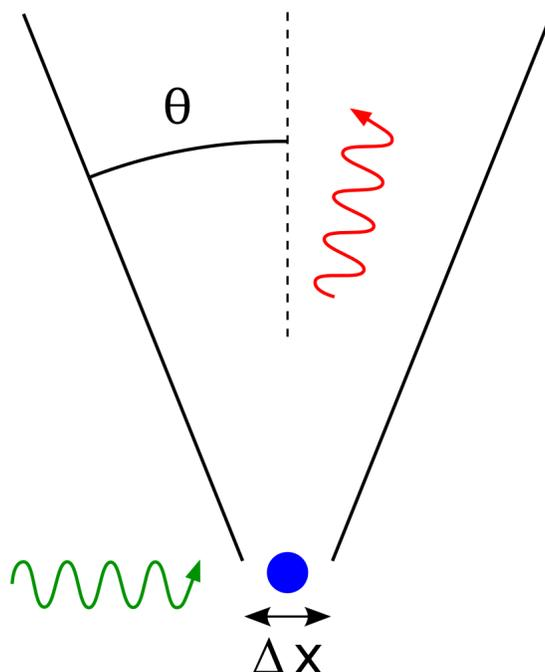
**Figure 1.1** Heisenberg's  $\gamma$ -ray microscope thought experiment. The incoming  $\gamma$ -ray (green) scatters against the electron (blue), producing a position measurement with the scattered  $\gamma$ -ray (red). The more precise the position measurement, the stronger the  $\gamma$ -ray disturbs the momentum of the electron.
