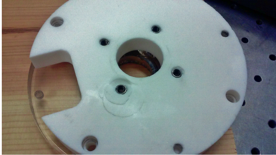
Figure 2.12: Fractured Macor ® insulating disk
