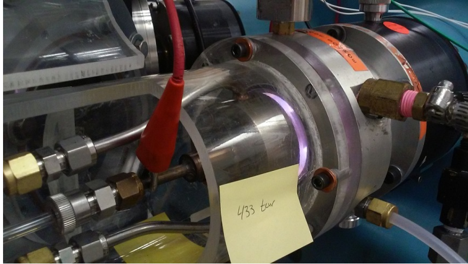
Figure 2.11: Picture of Hollow Cathode EUV source
