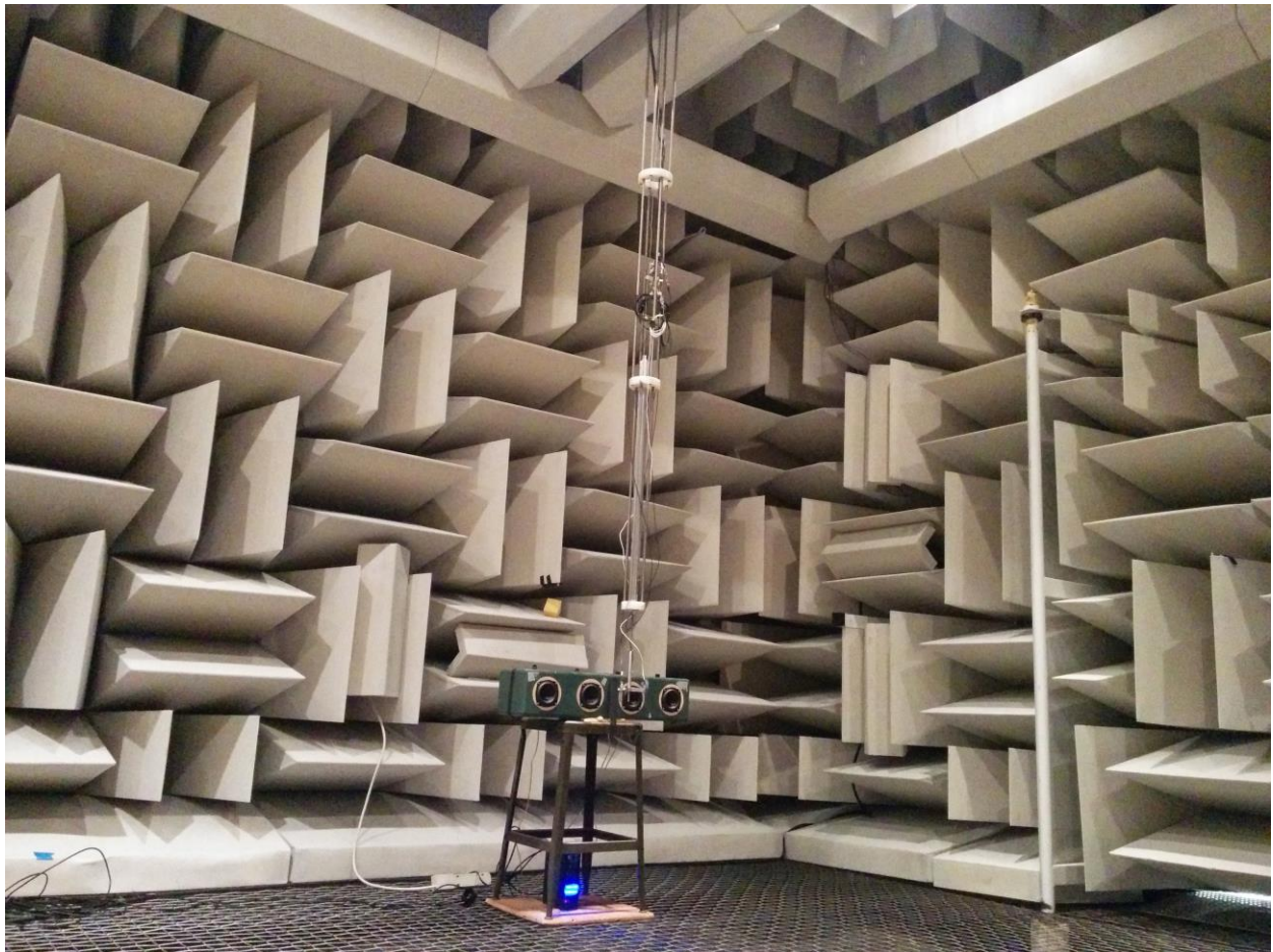
Figure 3 - The experimental setup in the corner of the large anechoic chamber at Brigham Young University. The intensity probe is suspended upside down form the boom arm that is hanging from the 3D precision positioning system. The plan to be scanned is directly in front of the loudspeaker array parallel to the floor.
