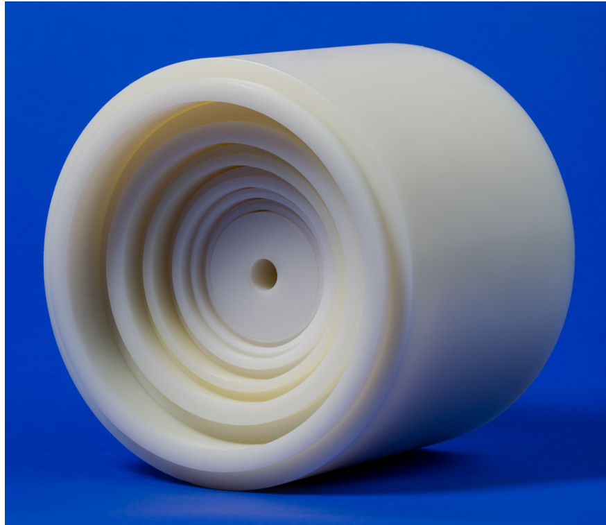
Figure 2.5 Moderating material from a nested neutron spectrometer (Nicholishiell 2013). Image used under the Creative Commons Attribution-Share Alike 3.0 Unported license.
