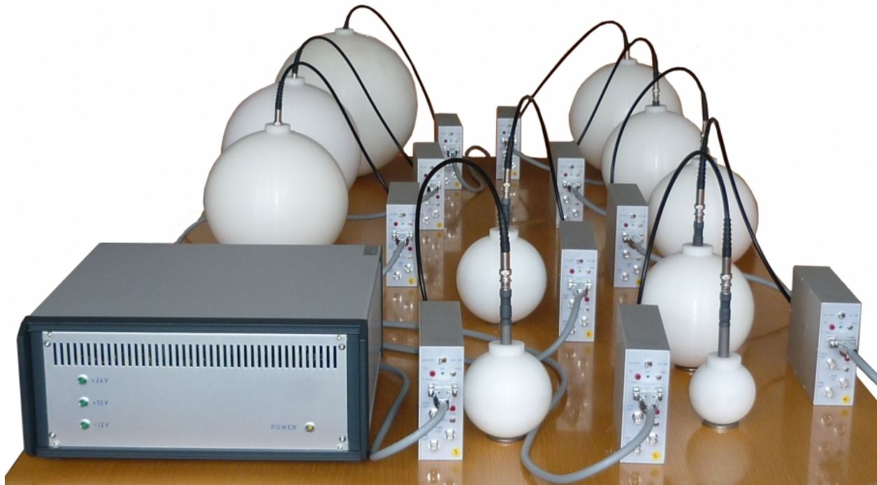
Figure 2.3 A Bonner sphere neutron spectrometer (ElseNuclear 2016).
