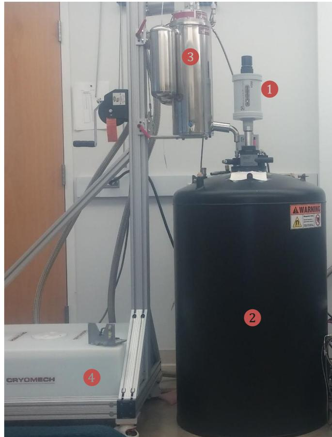
**Figure 1**—The PPMS and VSM setup. The VSM is located at position ①; samples are mounted through the top of the device and inserted inside the PPMS superconducting magnet, which is located at position ②. The pickup coils to perform VSM measurements are mounted before a sample is inserted. A CRYOMECH PT410 helium compressor is located at ③ to efficiently use the liquid helium needed for the superconducting components of the PPMS. A reservoir of liquid helium is located at ④.
