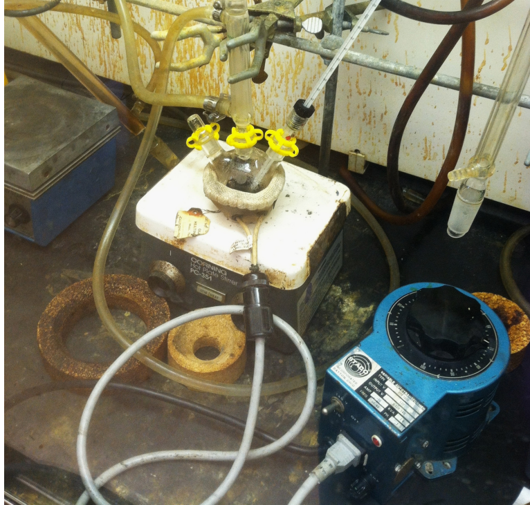
Figure 2.1 Image of our nanoparticle preparation. In this image the solution is being heated. Careful attention was given to temperature as this parameter controlled nanoparticle size.
