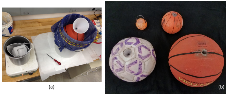
Figure 2.3 Pictures of making the source shielding, and the final product. We filled these balls with paraffin wax by melting several bars at a time over a hot plate and pouring the wax in the shell, shown in (a). We drilled a hole to the center in each, evident in (b). The source would be dropped in the sphere and data would be taken with the hole open at the top.
