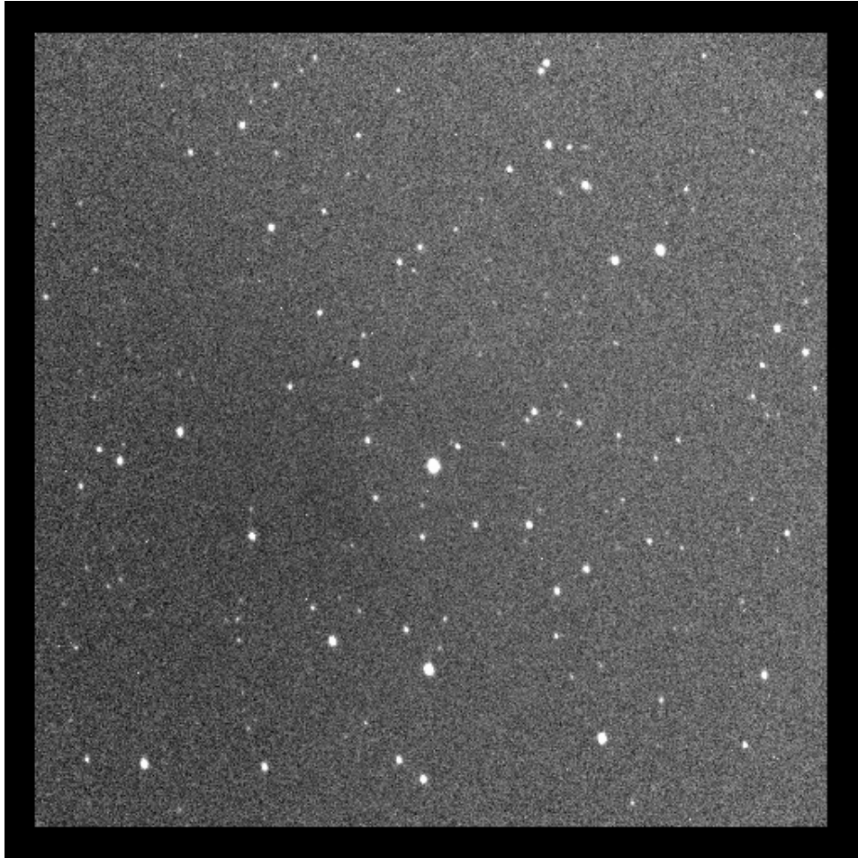
Figure 2.11 This is the final product of the DR script. This is one of many images that is now ready for photometry. The image should be a replica of when the Master Flat is divided out.
