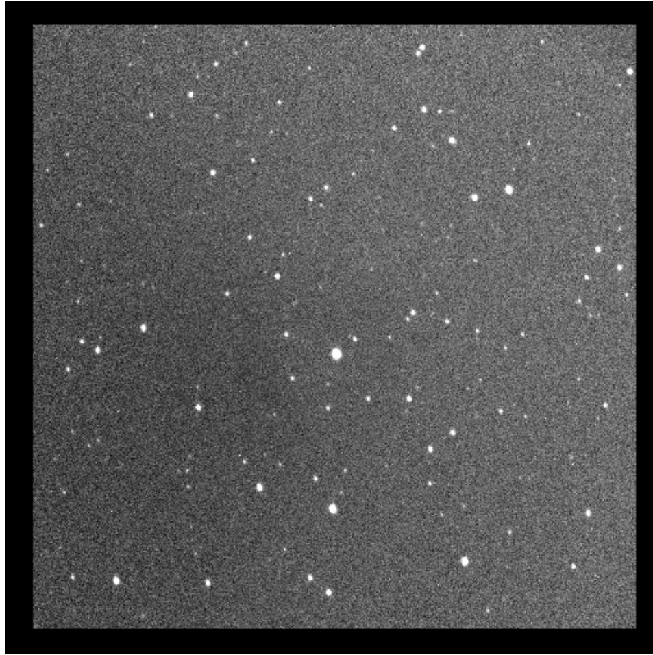
Figure 2.9 The Master Flat is divided out of the image after the Master Zero and Master Dark are subtracted out. This makes the illumination of the image uniform. The raw image is now completely data reduced and ready for photometry.
