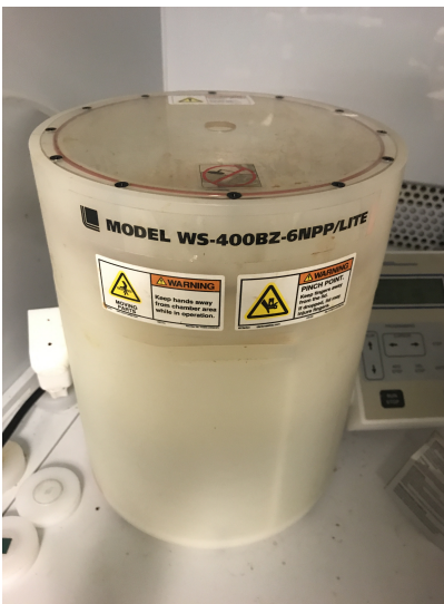
Figure 2.2 Photo resist spinner used to spin on PMMA
