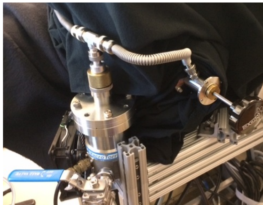
Figure 2.12 The third turbo is used to evacuate and pump down the two push rod handles. When the push rods are moved, it causes a temporary breach of vacuum, introducing unwanted contaminants and causing a spike in pressure. However constant pumping on the handles avoids that.
