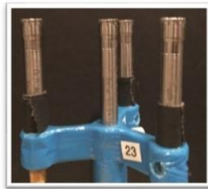
Figure 5: Probe C is an in-house built 2-dimensional intensity probe with ¼" microphones with d = 1 ".
