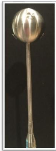
Figure 3: Probe A is a G.R.A.S. 3D Vector Probe Head Type 60LK.
