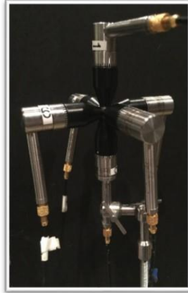
Figure 4: Probe B is a G.R.A.S. 50VI-1 Vector intensity probe.
