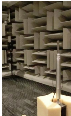
Figure 9: Photo showing a single reference microphone on the turntable with the loudspeaker in the corner of the anechoic chamber.
