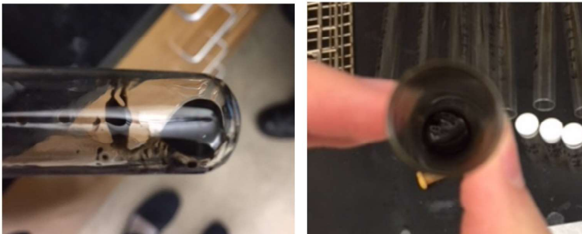
Figure 2.2 Nanoparticle solutions NP25 (left) and NP26 (right) after being centrifuged and decanted.
