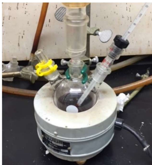
Figure 2.1 Heating mantle where the nanoparticles were held at 312° C for 30 min.
