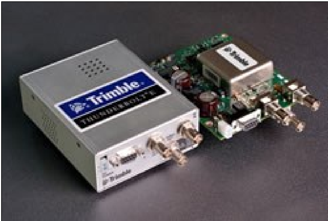
Illustration 1: Trimble Thunderbolt Disciplined GPS Receiver. This is used to further improve the long term accuracy of Rubidium clocks. Courtesy of Trimble Engineering. []
