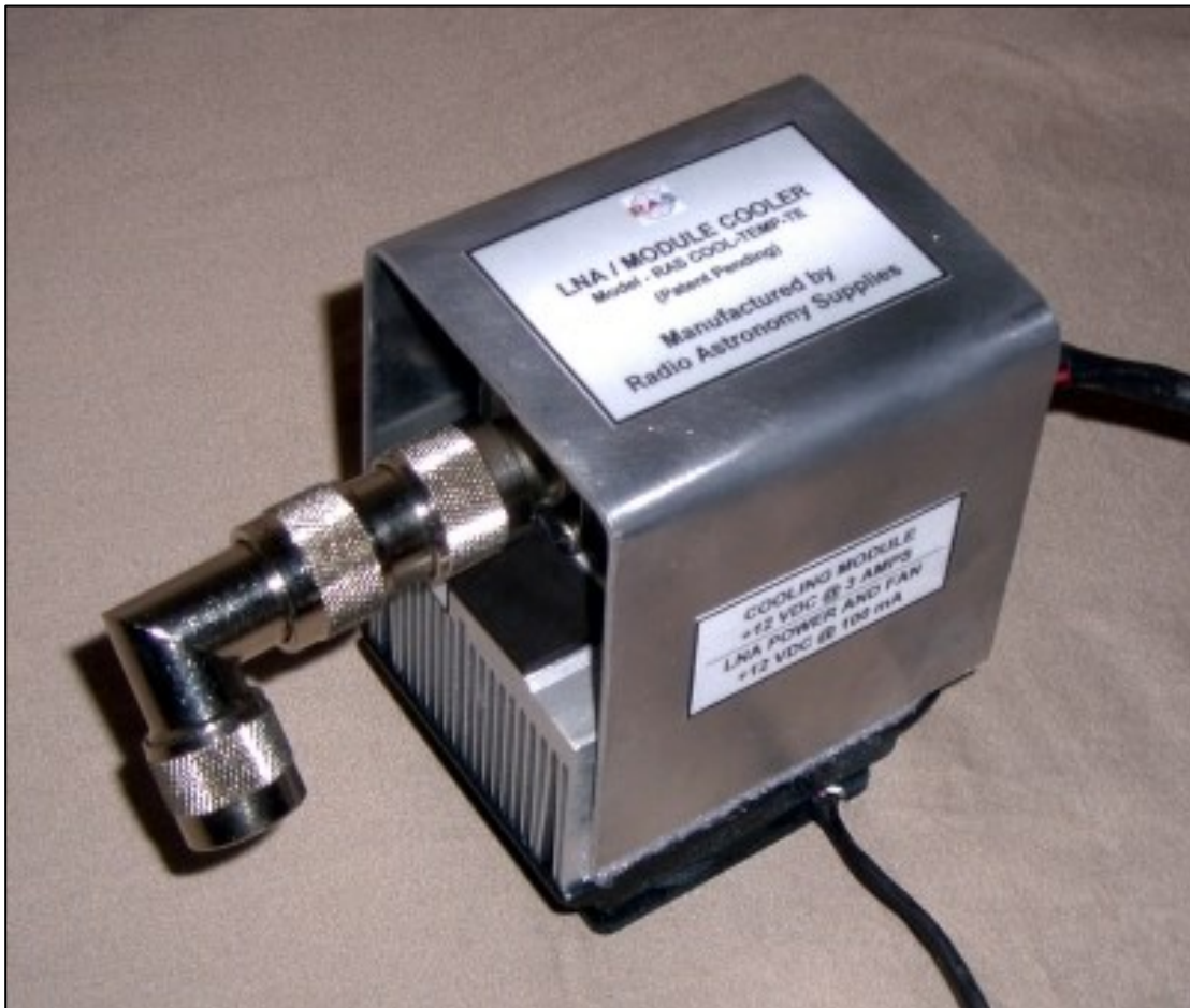
Figure 4-2: The Peltier Cooler - used to cool each LNA (by Radio Astronomy Supplies).
