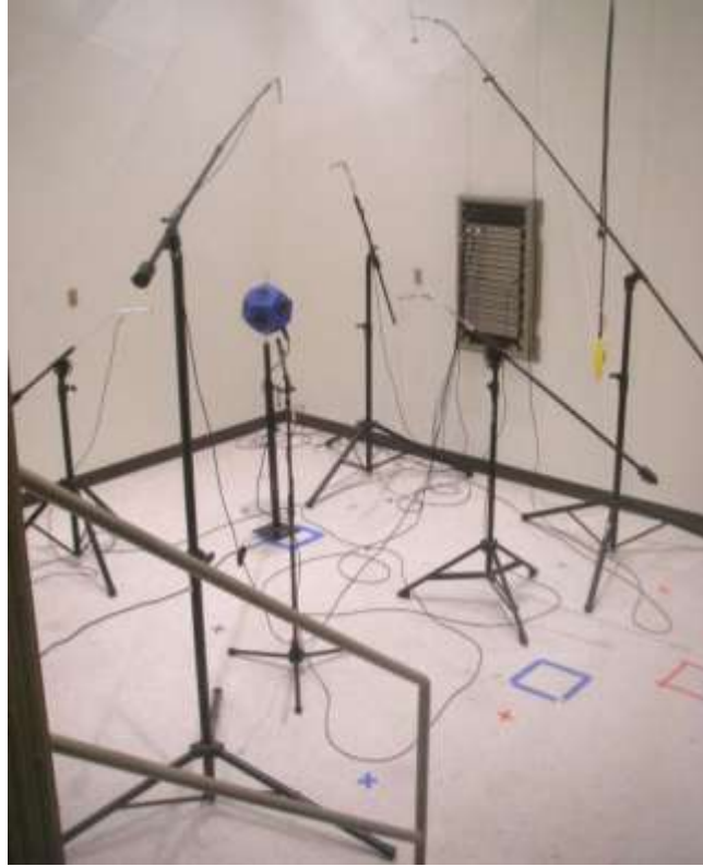
Figure 3.14 Test configuration for ISO 3741 in a reverberation chamber where some source-receiver distances have been deliberately set to less than the minimum distance d_{min} designated in the standard.
