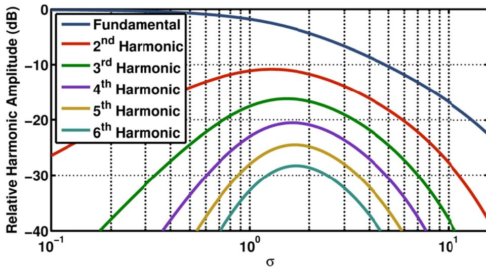
Figure 4.2. The first six harmonic amplitudes of waveforms predicted by numerically propagating an initially sinusoidal plane wave to various values of  $\sigma$  with thermoviscous losses. The amplitudes are plotted in dB relative to the amplitude of the initial signal. The Gol'dberg number of the source signal is 10.
