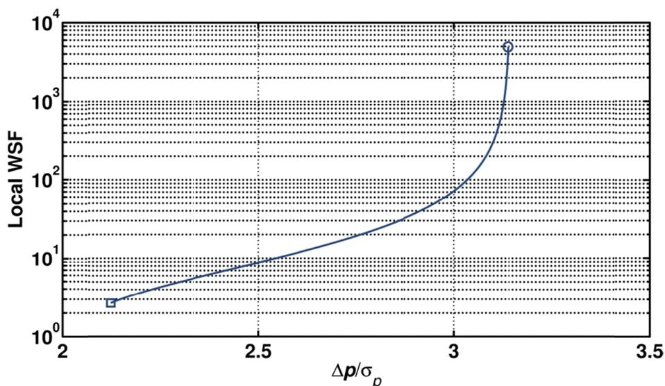
**Figure A.2. McInerny plot with ILWSF normalization locations for the Khokhlov solution. The locations are parametrically dependent upon  $\psi = (1 + \sigma)/\Gamma$ , where  $\sigma$  is the distance from the source over the shock formation distance and  $\Gamma$  is the Gol'dberg number. The circle denotes the location for  $\psi = 10^{-3}$ , and the square denotes the location for  $\psi = 4/3$ , and the line between the two are the locations for the values of  $10^{-3} > \psi > 4/3$ .**
