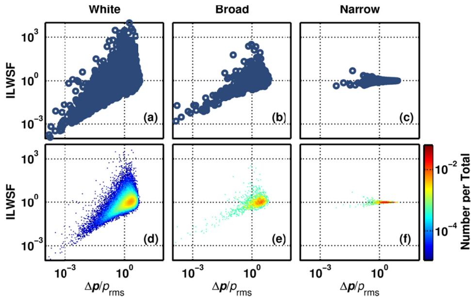
**Figure A.3.** McNerny plots of numerically generated spectrally (a) white, (b) broadband, and (c) narrowband Gaussian noise waveforms. The corresponding two-dimensional histograms are shown in plots (d), (e), and (f).
