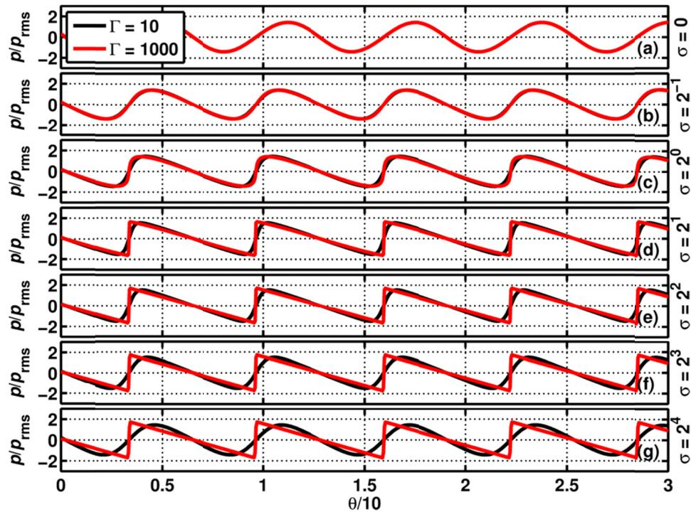
Figure 4.1. Portions of the waveforms predicted by numerically propagating an initially sinusoidal plane wave to various values of  $\sigma$  with thermoviscous losses and a Gol'dberg number of 10 (black lines) and 1000 (red lines).
