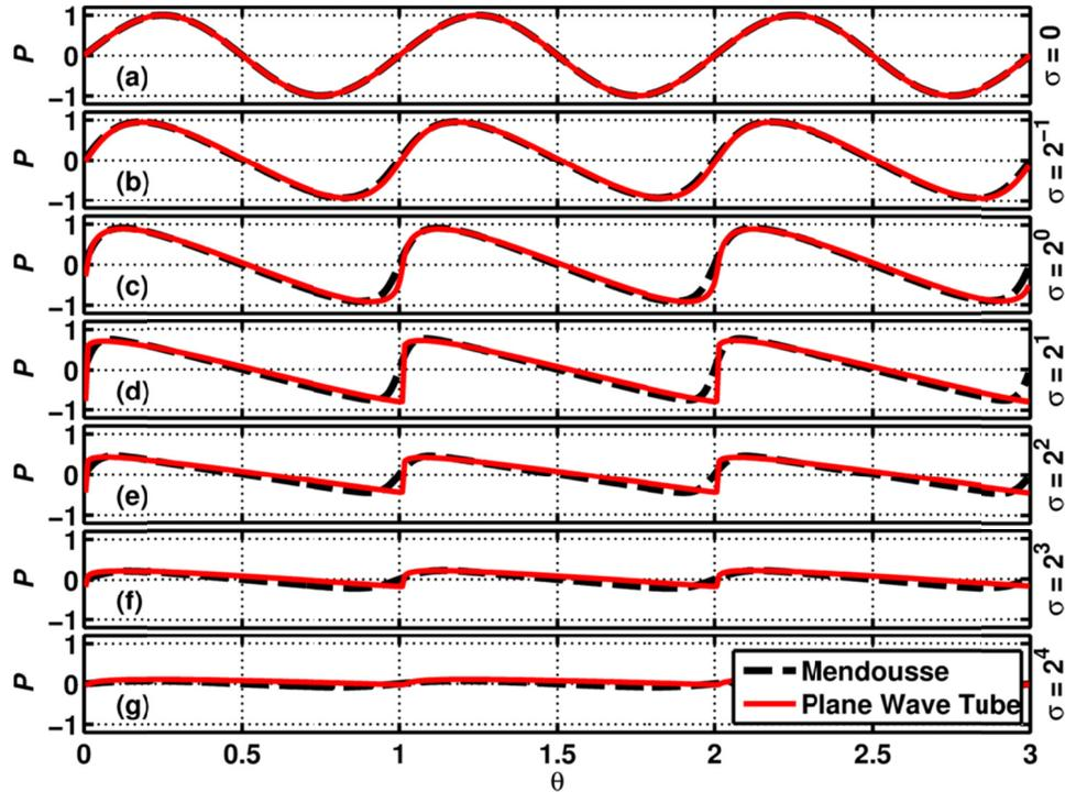
Figure 4.5. Portions of the waveforms predicted by numerically propagating an initially sinusoidal plane wave to various values of  $\sigma$  with linear losses similar to those of propagation in a plane wave tube (red), with the Mendousse solution (only thermoviscous absorption) plotted (dashed black), for comparison. The Gol'dberg number used for this plot is 10.
