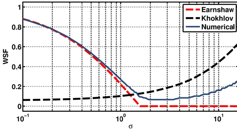
**Figure 4.7.** Estimates of the wave steepening factor (WSF) of waveforms predicted by numerically propagating an initially sinusoidal plane wave to various values of  $\sigma$  with linear losses similar to those of propagation in a plane wave tube.
