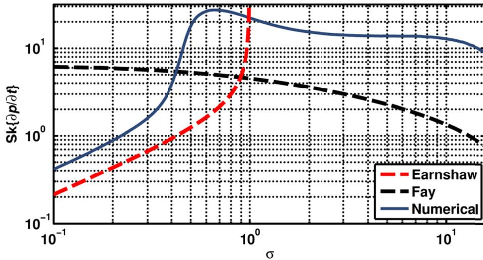
Figure 4.12. Estimates of the derivative skewness of waveforms predicted by numerically propagating an initially broadband plane wave to various values of  $\sigma$  with linear losses similar to those of propagation in a plane wave tube.
