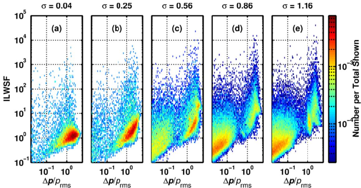
**Figure A.10.** Portions of the histograms of the McNerny plots of initially 1500 Hz broadband noise with jet noise-like statistics measured in a plane wave tube (a) 0.3 m, (b) 2.5 m, (c) 5.6 m, (d) 8.6 m, and (e) 11.6 m from the source.
