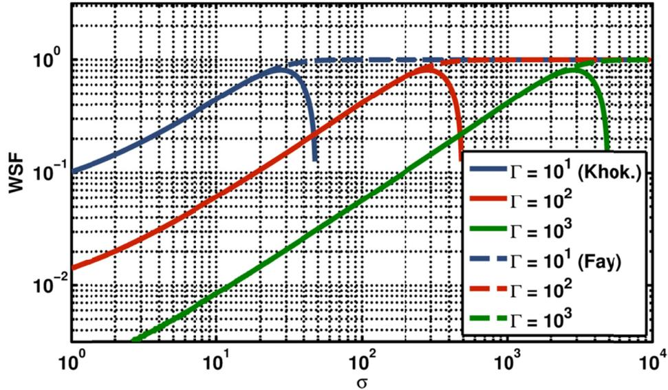
Figure 3.2. Plot of the wave steepening factor found using the Khokhlov solution (Khok.) and using the Fay solution, both plotted as a function of  $\sigma$  for three different values of Gol'dberg number.
