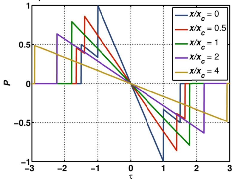
**Figure 1.1.** An example of shock propagation and coalescence. The source waveform is a double N-wave, and the propagation does not include linear losses. Weak shock theory and the Earnshaw solution were used to predict the propagation. At  $x = x_c$  the two positive shocks merge, as do the two negative shocks.
