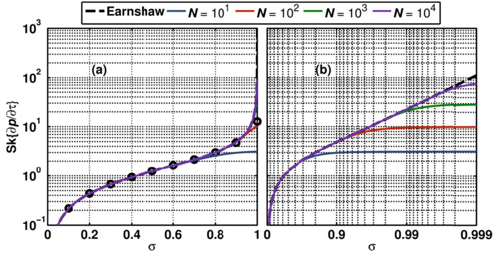
Figure 3.4. The analytical derivative skewness of an initially sinusoidal waveform modeled by the Earnshaw solution and estimates of the derivative skewness of the Fubini solution using  $N$  terms of each of the infinite series in Equation (3.55). The derivative skewness values are plotted on (a) a linear abscissa and (b) a logarithmic abscissa. The derivative skewness values found by Shepherd *et al.* [37] are plotted (black circles) in (a), for comparison.
