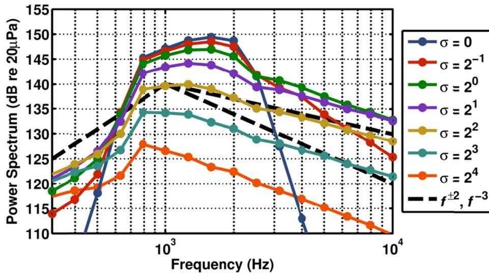
Figure 4.10. One-third octave power spectra predicted by numerically propagating an initially broadband Hz plane wave to various values of  $\sigma$  with linear losses similar to those of propagation in a plane wave tube.
