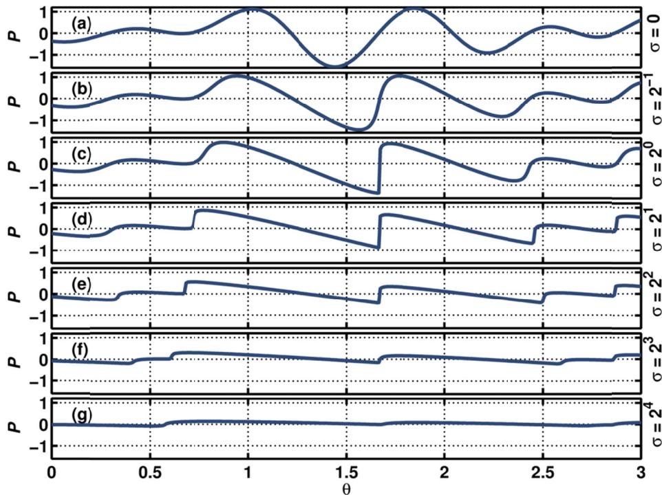
**Figure 4.9.** Portions of the waveforms predicted by numerically propagating an initially broadband Hz plane wave to various values of  $\sigma$  with linear losses similar to those of propagation in a plane wave tube.
