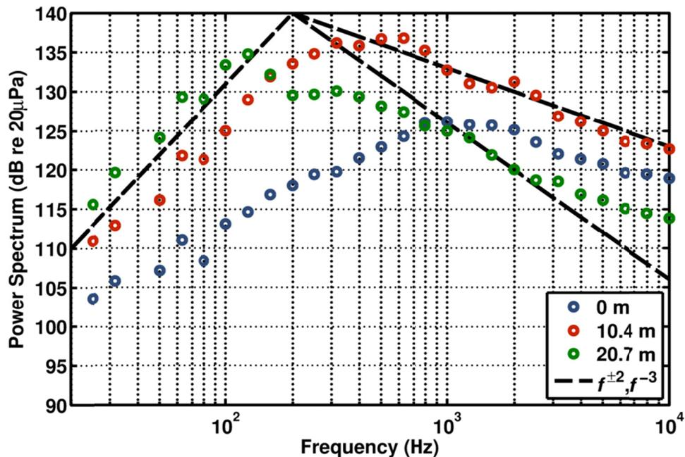
Figure 6.5. One-third octave band power spectra of waveforms measured 0 m, 10.4 m, and 20.7 m downstream of an F22-A Raptor at military engine condition. The dashed lines represent  $f^{+2}$  and  $f^{-3}$  dependencies.
