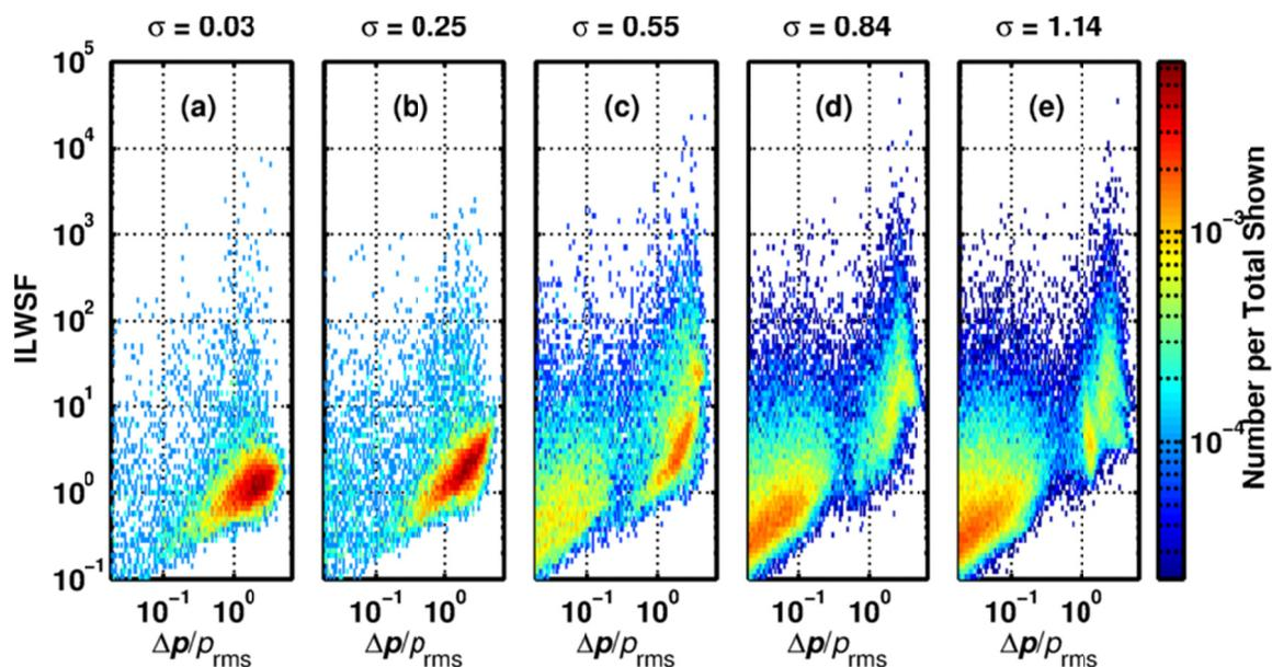
Figure A.6. Portions of the histograms of the McInerny plots of initially 1500 Hz broadband Gaussian noise measured in a plane wave tube (a) 0.3 m, (b) 2.5 m, (c) 5.6 m, (d) 8.6 m, and (e) 11.6 m from the source.
