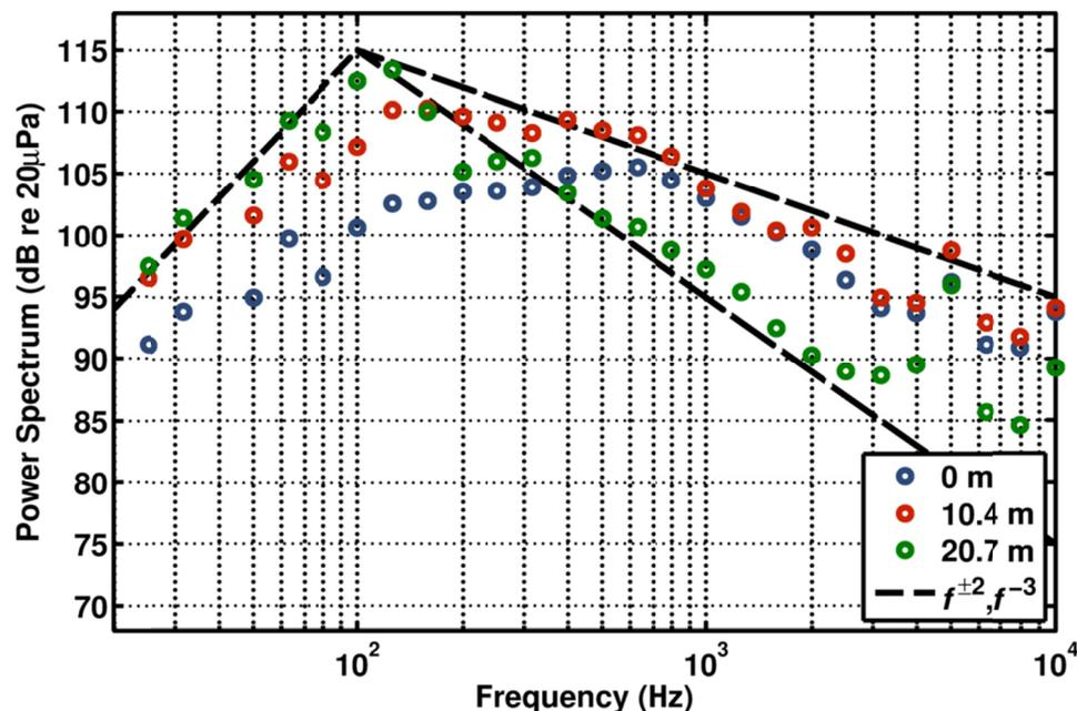
Figure 6.4. One-third octave band power spectra of waveforms measured 0 m, 10.4 m, and 20.7 m downstream of an F22-A Raptor at intermediate engine condition. The dashed lines represent  $f^{+2}$  and  $f^{-3}$  dependencies.
