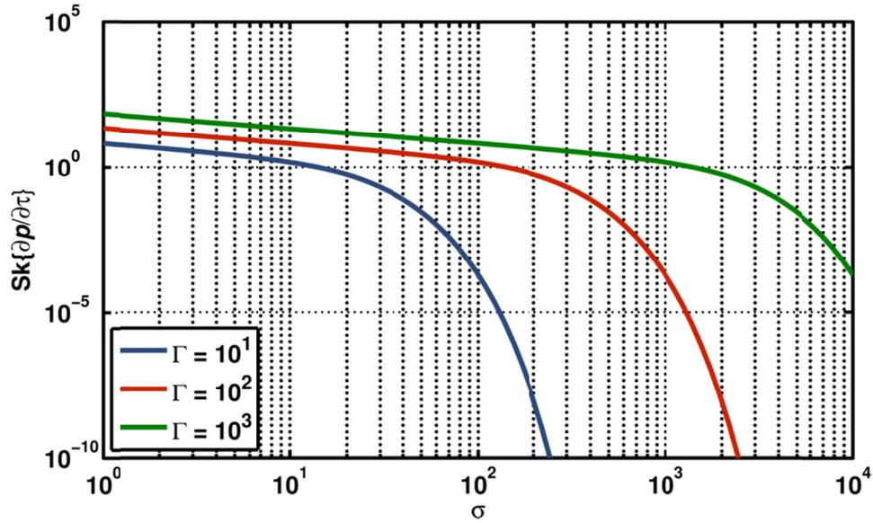
Figure 3.5. The skewness of the time-derivative of the pressure (derivative skewness, or  $\text{Sk}\{\partial p/\partial\tau\}$ ) of the Fay solution as a function of  $\sigma$  for three values of Gol'dberg number.
