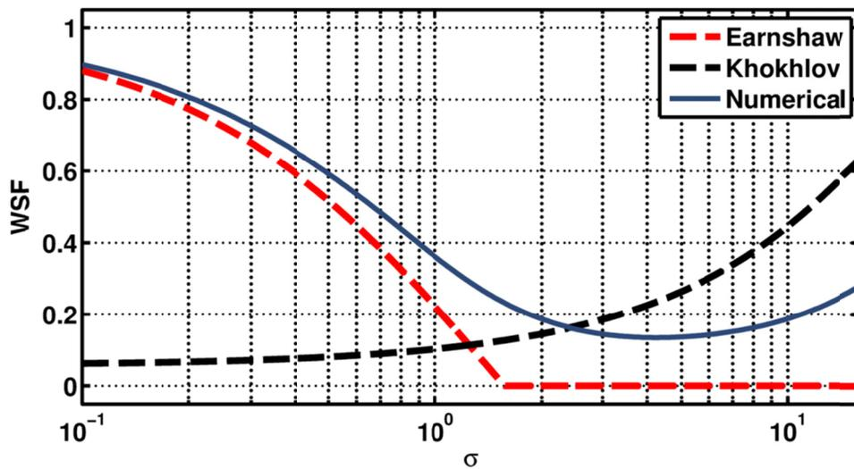
Figure 4.11. Estimates of the wave steepening factor (WSF) of waveforms predicted by numerically propagating an initially broadband plane wave to various values of  $\sigma$  with linear losses similar to those of propagation in a plane wave tube.
