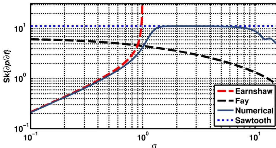
Figure 4.8. Estimates of the derivative skewness of waveforms predicted by numerically propagating an initially sinusoidal plane wave to various values of  $\sigma$  with linear losses similar to those of propagation in a plane wave tube. The dotted blue line represents the upper limit based on a discretely sampled sawtooth wave.
