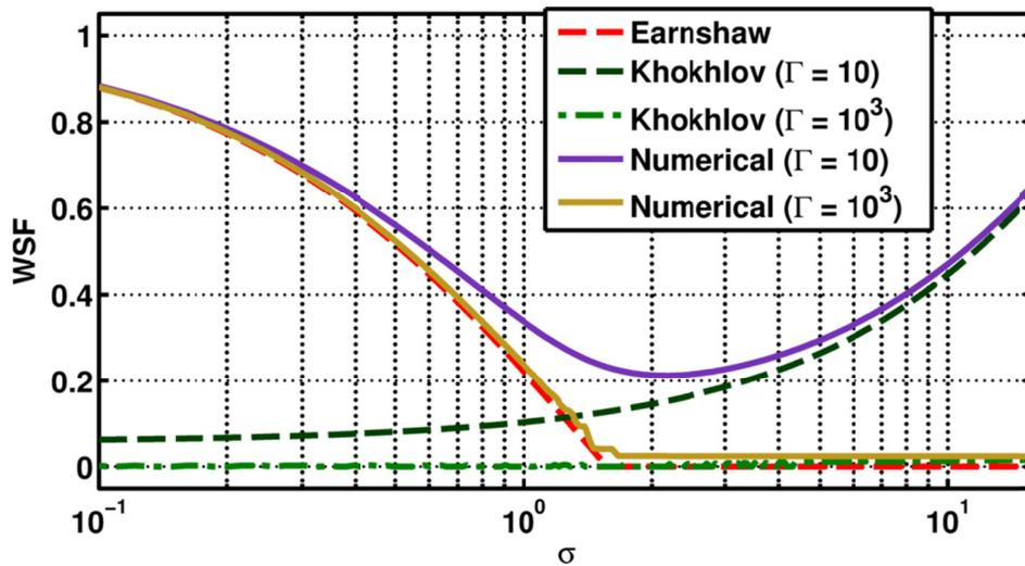
**Figure 4.3.** Estimates of the wave steepening factor (WSF) of waveforms predicted by numerically propagating an initially sinusoidal plane wave to various values of  $\sigma$  with thermoviscous losses.
