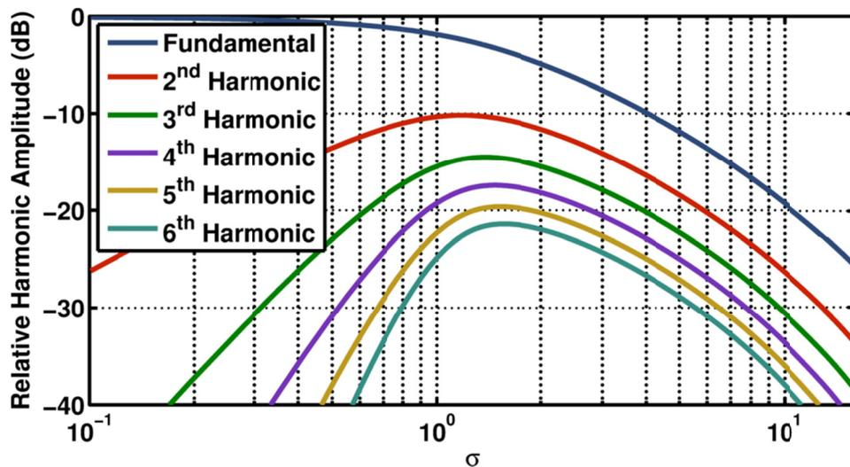
Figure 4.6. The first six harmonic amplitudes of waveforms predicted by numerically propagating an initially sinusoidal plane wave to various values of  $\sigma$  with linear losses similar to those of propagation in a plane wave tube. The Gol'dberg number used for this plot is 10.
