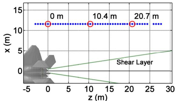
**Figure 6.1.** Schematic of the measurement locations, relative to the aircraft, used during the July 2009 measurement of noise radiating from an F-22A Raptor. The blue dots represent a fixed array of reference microphones set on the ground. The three circled microphone locations are microphones that are specifically referenced in the text.
