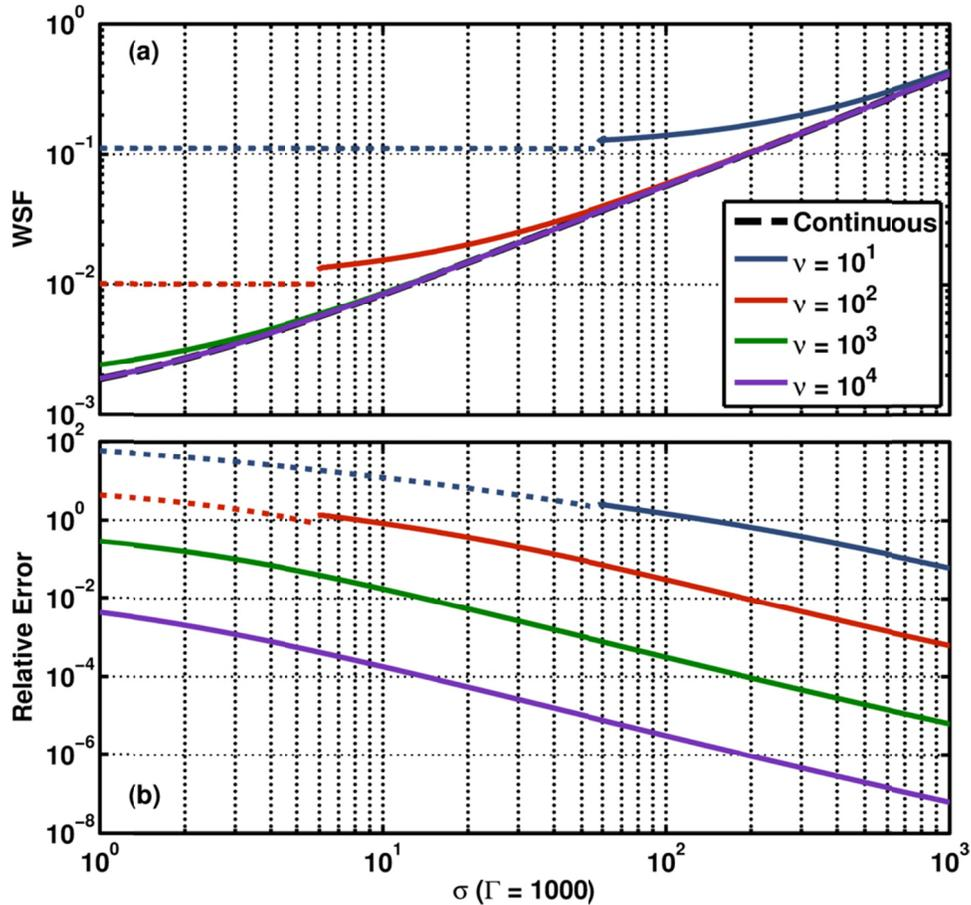
Figure 3.7. (a) Estimates of the wave steepening factor (WSF) of the Khokhlov solution for  $\nu = 10^1, 10^2, 10^3$ , and  $10^4$ . The dashed lines denote the WSF of a sawtooth wave. The exact WSF derived from using continuous sampling is plotted as the black dashed line, for comparison. (b) The relative error of the estimates in (a). The relative error is defined as  $|1 - \text{WSF}_\nu / \text{WSF}_{\text{cont}}|$ .
