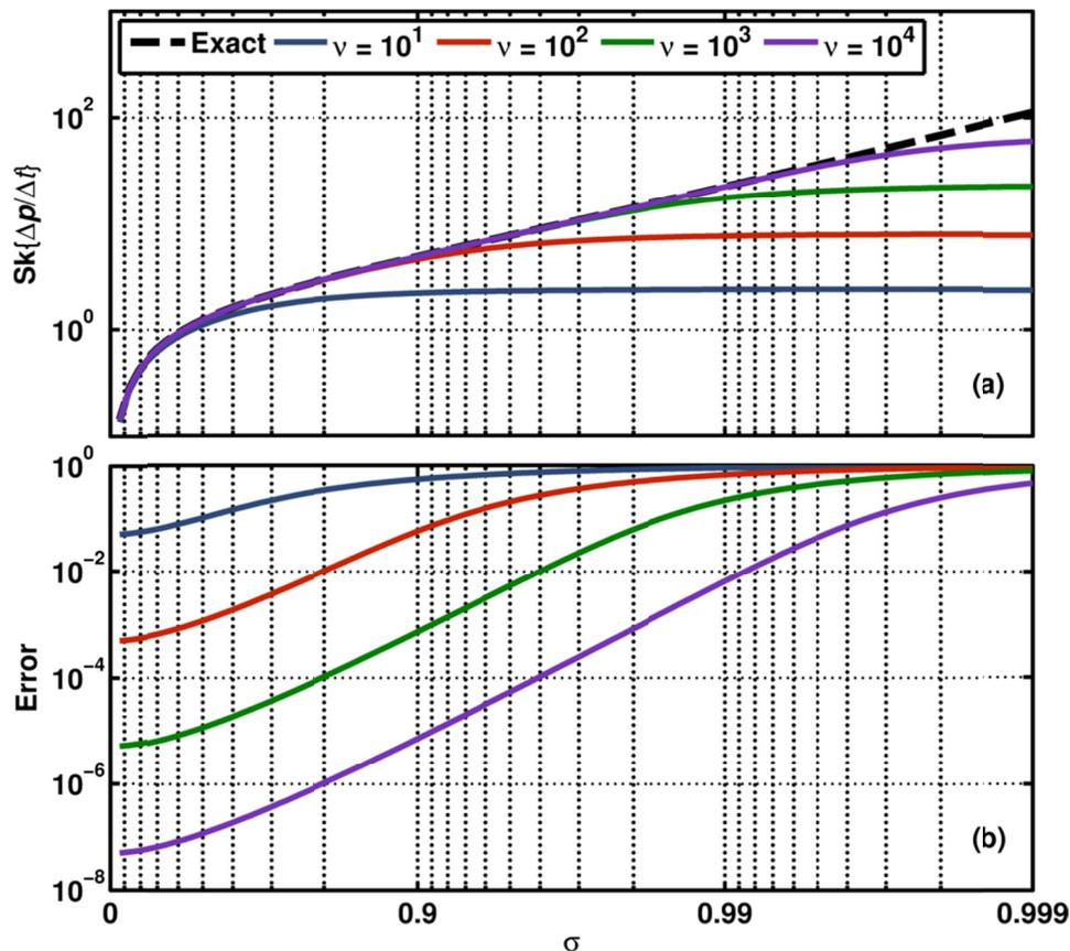
Figure 3.8. (a) Estimates of the derivative skewness of the Fubini solution for  $\nu = 10^1$ ,  $10^2$ ,  $10^3$ , and  $10^4$ . The exact derivative skewness derived from using continuous sampling is plotted for comparison. (b) The relative error of the estimates in (a). The relative error is defined as  $|1 - Sk\{\Delta P/\Delta\theta\}/Sk\{\partial P/\partial\theta\}|$ , where the  $\Delta$ 's indicate discrete sampling and the  $\partial$ 's indicate continuous sampling.
