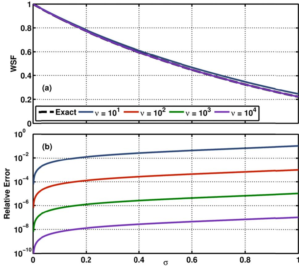
Figure 3.6. (a) Estimates of the WSF for  $\nu = 10^1, 10^2, 10^3$ , and  $10^4$ . The exact WSF derived from using continuous sampling is plotted for comparison. (b) The relative error of the estimates in (a). The relative error is defined as  $|1 - \text{WSF}_\nu / \text{WSF}_{\text{cont}}|$ , where  $\text{WSF}_\nu$  is the estimate of the WSF for a given value of  $\nu$ , and  $\text{WSF}_{\text{cont}}$  is the exact WSF value using continuous sampling.
