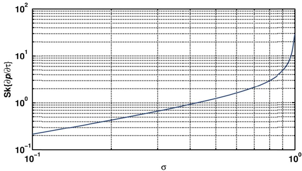
Figure 3.3. The skewness of the time-derivative of the pressure (derivative skewness, or  $\text{Sk}\{\partial p/\partial \tau\}$ ) of the Fubini solution. The dimensionless variable  $\sigma$  is the distance from the source divided by the shock formation distance.
