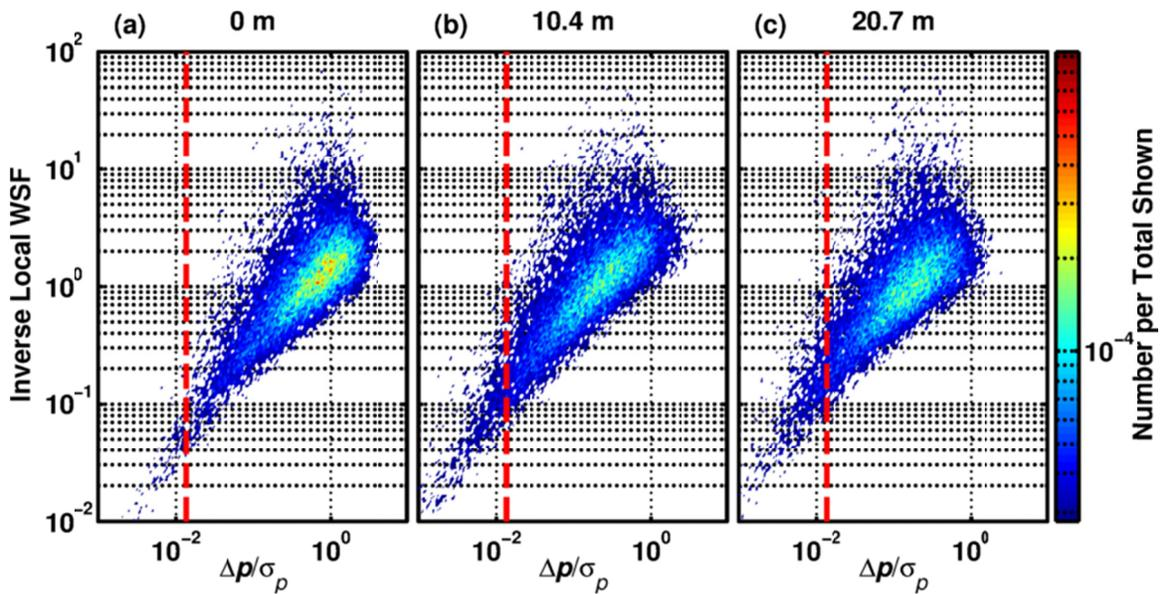
Figure A.12. Two-dimensional histograms of McInerny plots with ILWSF normalization of noise waveforms measured on the ground array (a) 0 m, (b) 10.4 m, and (c) 20.7 m downstream of the nozzle of an F22-A Raptor at military engine condition. The red dashed line represents the threshold suggested by McInerny and Ölçmen.
