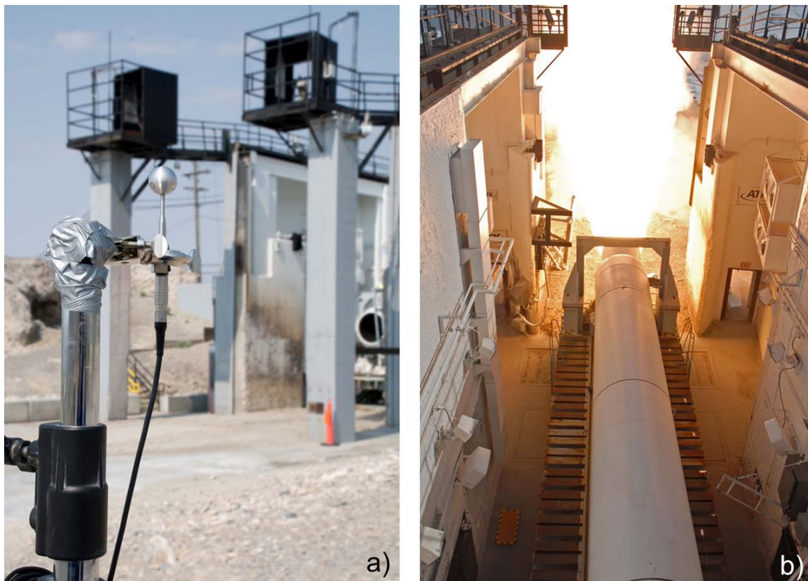
Figure 6.1. Two views of a GEM-60 solid rocket motor a) from the point of view of a SA array downstream (rocket nozzle is in the background) and b) during firing as viewed from above.
