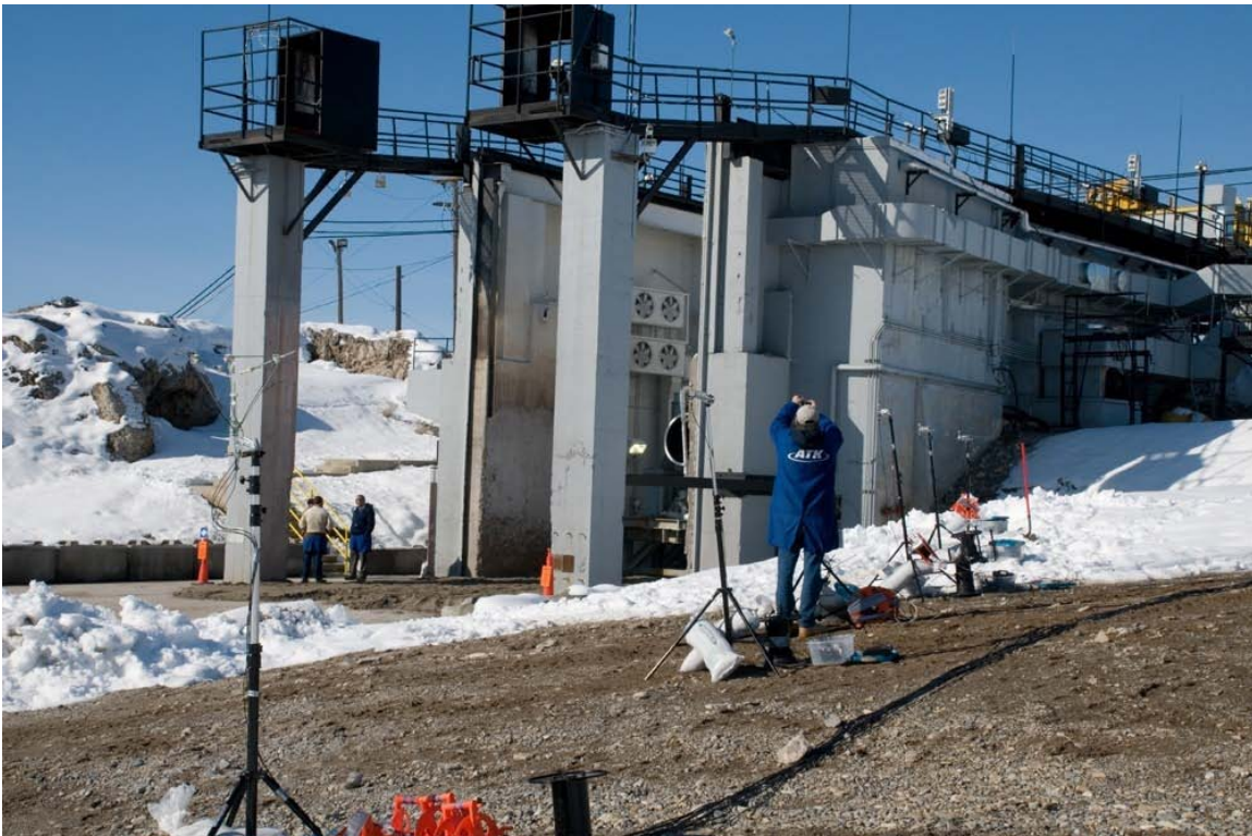
Figure 6.2. A line of microphone arrays is set parallel to the shear layer of a GEM-60 solid rocket motor in preparation for the February 2009 test firing.
