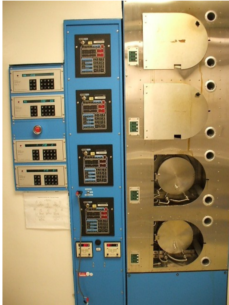
Figure 2-2 Canary furnace used for LPCVD of low stress silicon nitride
