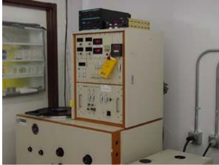
Figure 2-4 Anelva RIE DEM-451 used for Reactive Ion Etching
