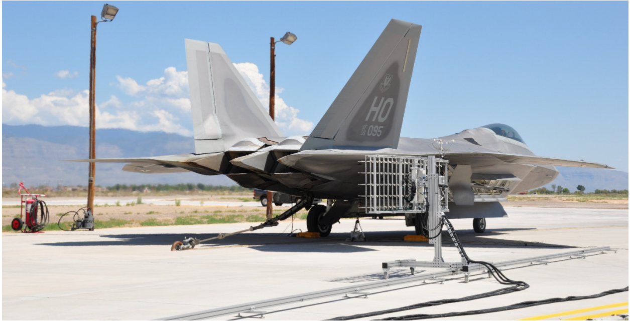
Figure 2.1 F-22A and 90-microphone array on adjustable-height rig. During engine cool-down, the rig was moved along the guide rail to 10 locations downstream.
