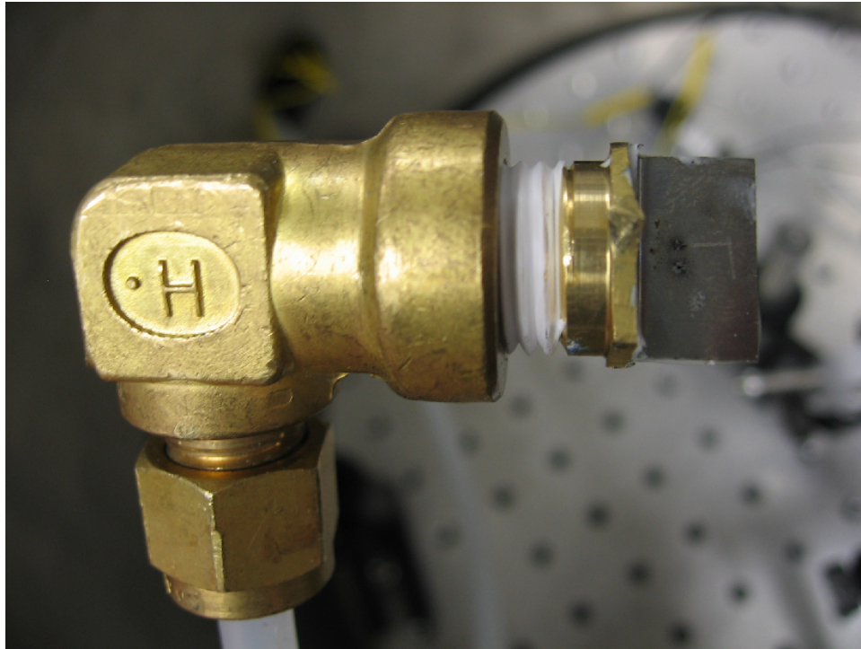
Figure 3.9 Example of Gas Cell with the two drilled holes for the beam paths
