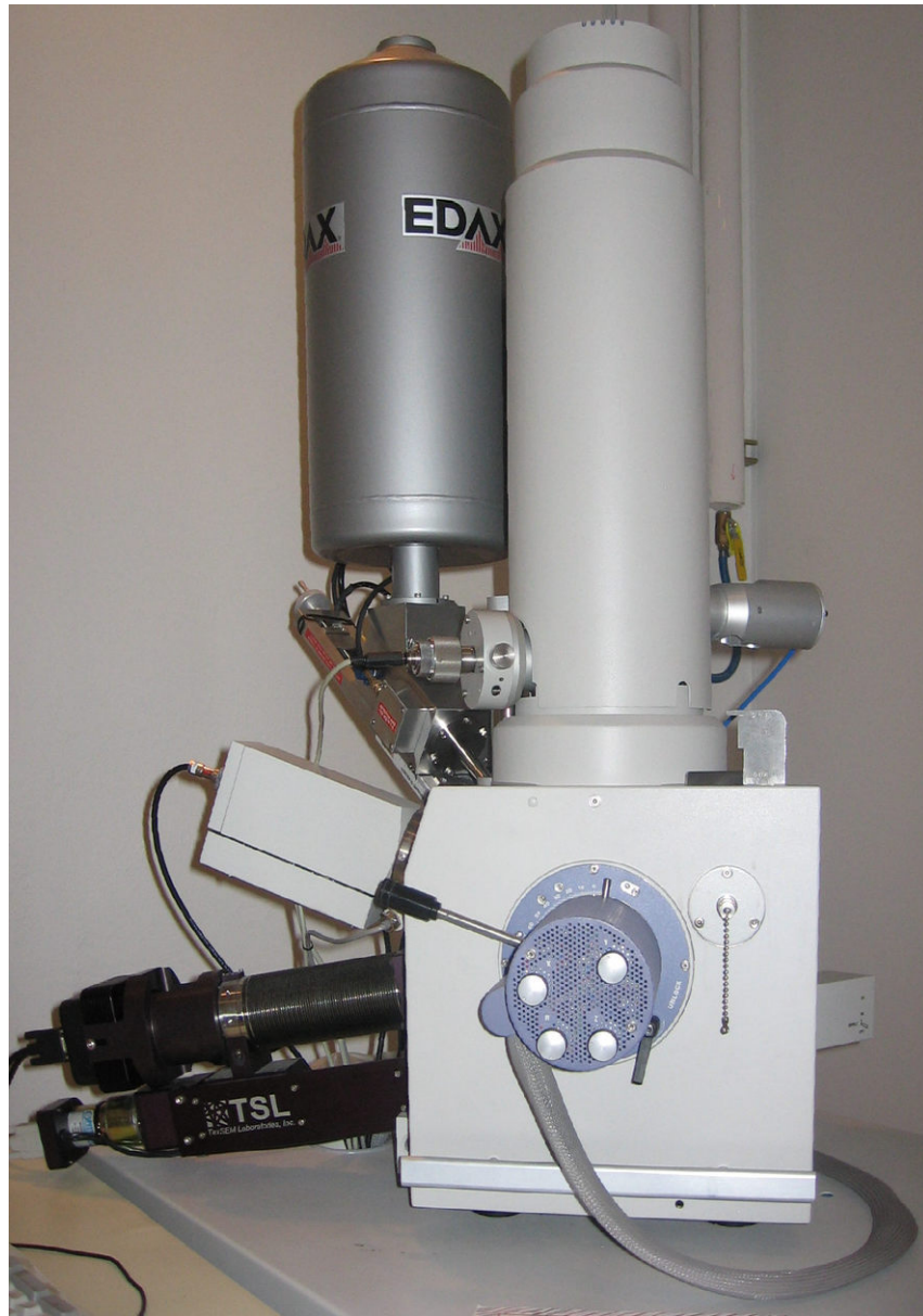
Figure 4.8 Phillips XL30 Scanning Electron Microscope. Shown in the picture are also the SE, the XEDS, and the EBSD detectors
