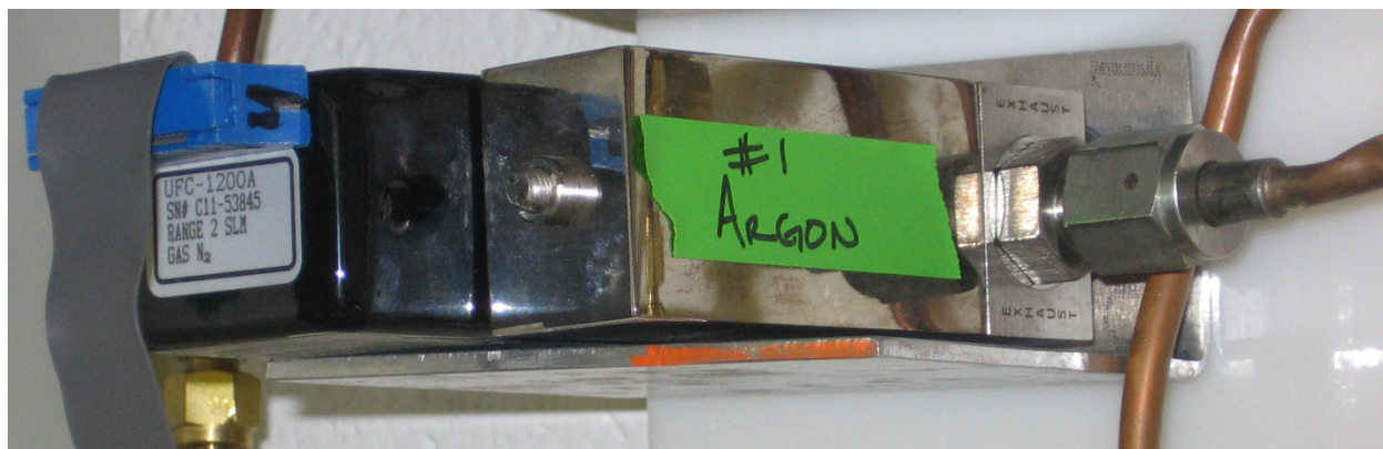
Figure 4.7 Mass Flow Controller used to control the argon flow.
