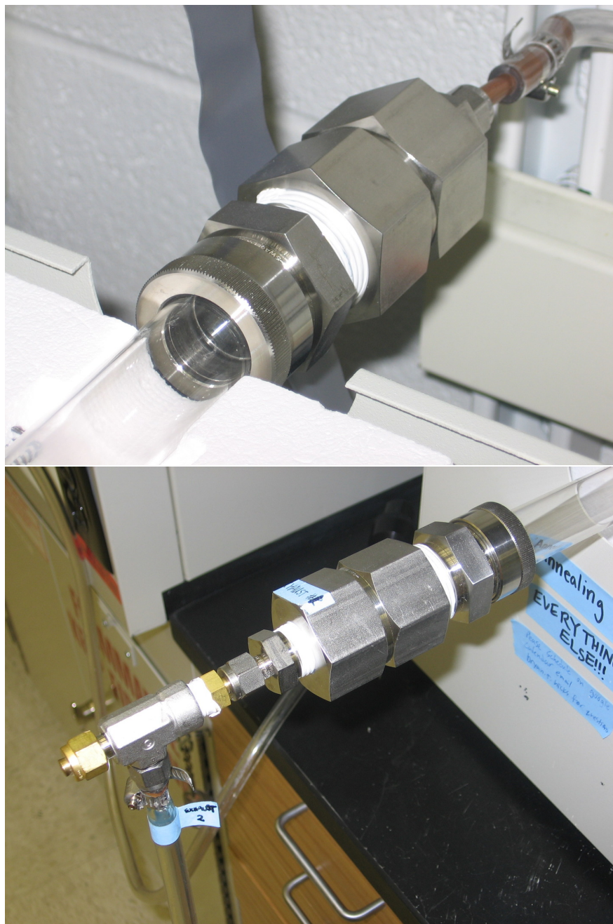
Figure 4.6 Both inlet and outlet to the quartz tube are fitted with a rubber “O”-ring to form an air-tight seal. Further, the outlet was outfitted with a “T” joint to allow a guiding rod to move the sample into and out of the “hot-zone.” (Here, the “T” joint is plugged as it is not being used)
