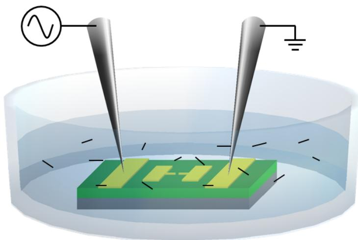
**Figure 1.4** A cartoon image of the setup used in FPD experiments. The AC driving signal localizes nanotubes between the floating electrodes at the center of the image. Just like the cereal box, the CNTs are enlarged to show texture.
