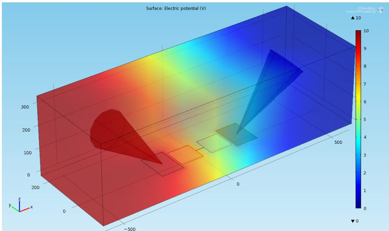
**Figure 4.7** Finite Element Analysis simulation of the potential surrounding the geometry 1 system. It is clear to see the gradient in fluid potential between the driving electrodes and that the potential on the FEs is held by a sort of "weighted average" of the fluid potential immediately above them.
