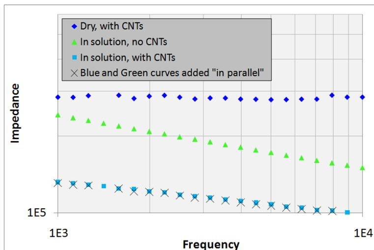
**Figure 4.3** A zoomed in portion of the data presented in figure 3.7. The X's mark calculated data points of adding the dry measurement of CNTs in parallel with the measurement of electrodes in solution without CNTs. The agreement of this calculation with the measured data indicates that these measurements are valid and that the CNTs can cause large changes in impedance between the FEs as they are localized.
