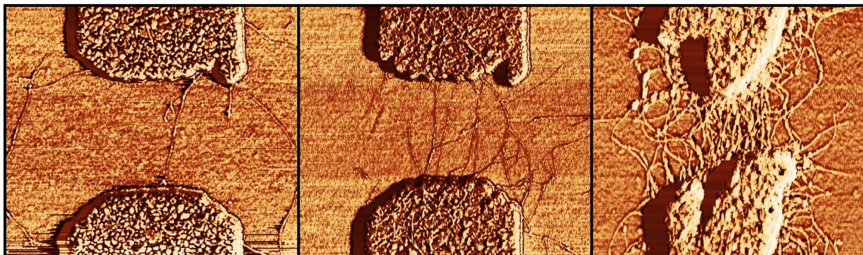
**Figure 3.4** AFM phase images of geometry 5 devices with 1  $\mu\text{m}$  wide FE fingers. While the devices with smaller FE fingers shown in figure 3.3 captured at most 4 CNTs, these larger devices often captured many more CNTs. Depending on the voltage and FE size, anywhere from 0 to 33 CNTs were observed captured in these larger devices. Images are 2  $\mu\text{m}$  wide on a side. Irregularities in electrode shape were due to writing glitches during electron-beam lithography exposure.
