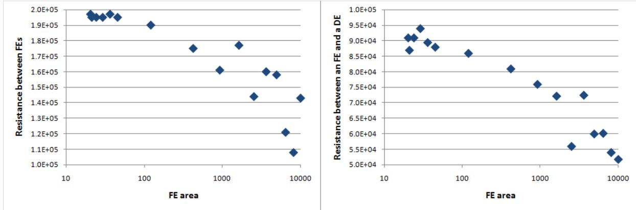
**Figure 3.8** Measured resistance between an FE and a DE (left) and between FEs (right) as a function of FE area. The geometry of figure 2.3 was used for these measurements. This data indicates that as FE area decreases, the resistance between the various electrodes increases.
