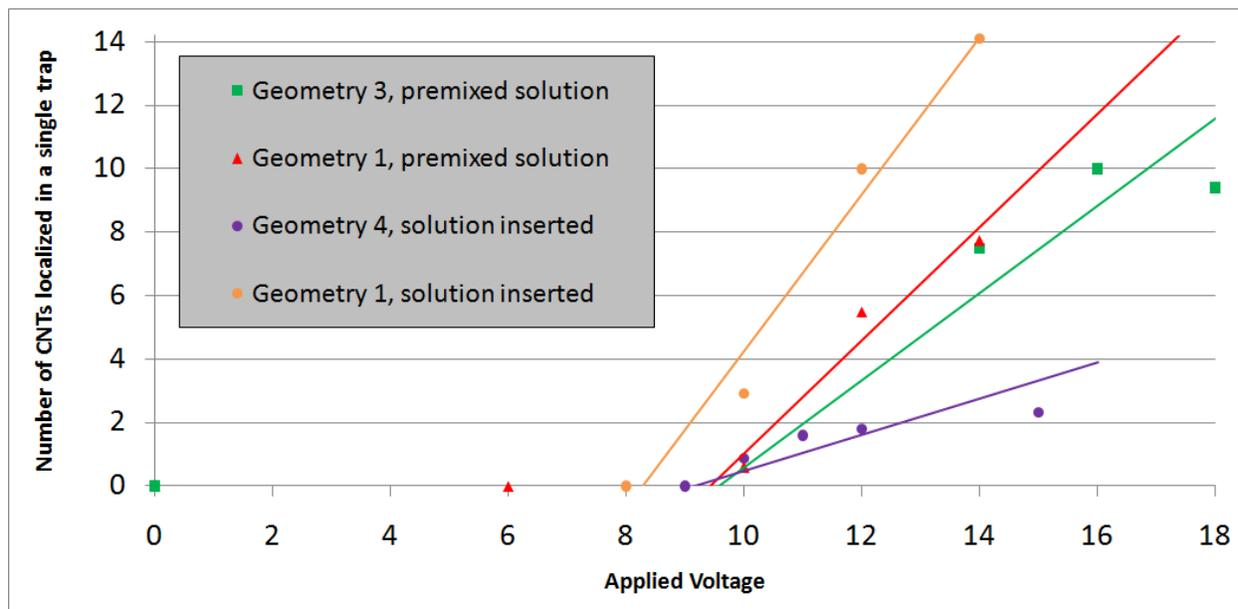
**Figure 3.1** Comparison of the two methods of FPD used in this study: when the CNT suspension was added to the die in a dish of water, and when the suspension was diluted in water and added to dry electrodes. Each data point represents an average of  $\sim 10$  devices. Error bars have been omitted for clarity.
