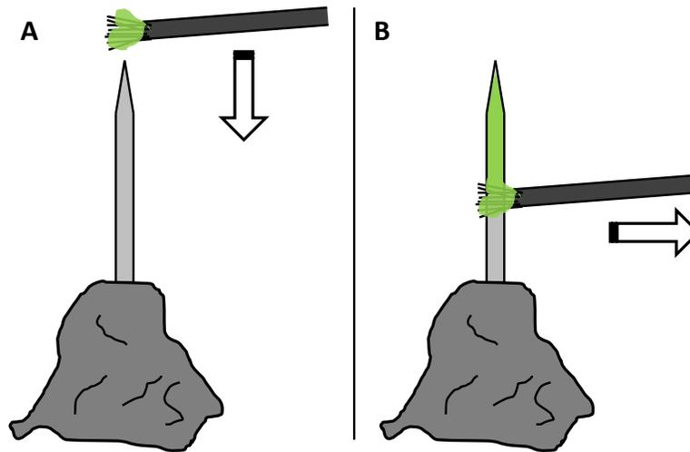
**Figure 2.4** A) Needles were pressed into a stand made of aluminum foil and the nail polish brush lowered directly through the needle apex. B) The brush was removed horizontally. The sharpness of the needle apex caused the polish to wick away, leaving a very small region of the apex uncoated.
