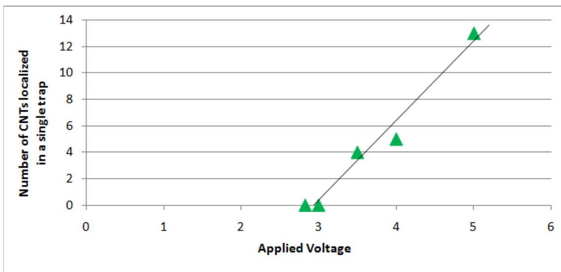
**Figure 3.2** Results of experiments applying a voltage directly to  $100 \mu\text{m}$  square FEs, using the geometry of figure 2.3. This behavior is very similar to the results of FPD on these FEs (see figure 3.1), but the voltage threshold was much lower and the slope nearly three times steeper.
