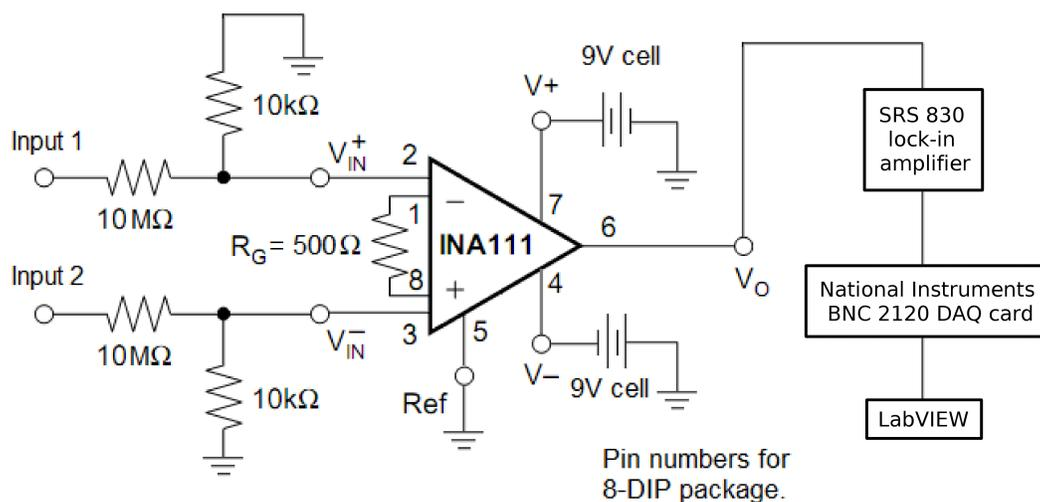
**Figure 2.8** Schematic for high input impedance AC potentiometer.
