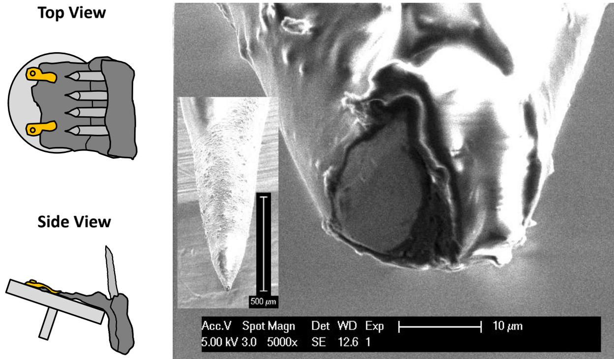
**Figure 2.5** Left: Cartoon image showing how the needles were mounted to position and stabilize them for SEM imaging. The aluminum foil basket both served as a carrying case as well as conductive medium to ground the needles during imaging for high contrast. In this way the exposed conductive region of the needle could be easily seen through the insulating nail varnish. Right: SEM micrograph of a micromanipulator probe insulated at all but the apex.
