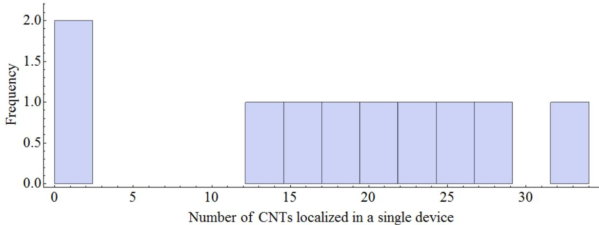
**Figure 4.1** Histogram of data showing the number of CNTs localized in each trap when DEP was performed for 540 s, the average of which forms one of the data points in figure 3.6 A. The data is distributed fairly evenly around the average of 22 localized CNTs, except for the two devices which captured an unusually low number of CNTs at the left.
