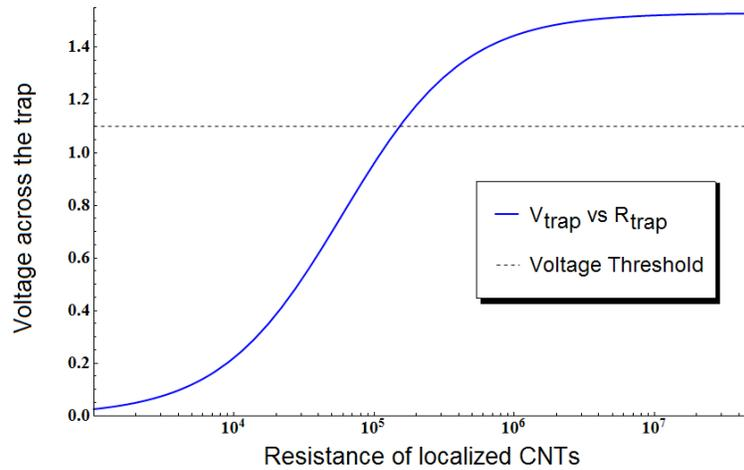
**Figure 4.5** Plot of equation 4.3 with respect to  $R_{trap}$  capacitance and resistance values measured using the geometry of figure 2.6. As a device localizes CNTs  $R_{trap}$  decreases. Once  $R_{trap}$  is sufficiently low  $|V_{trap}|^2$  (proportional to the dielectrophoretic force) is small and the device no longer attracts tubes.
