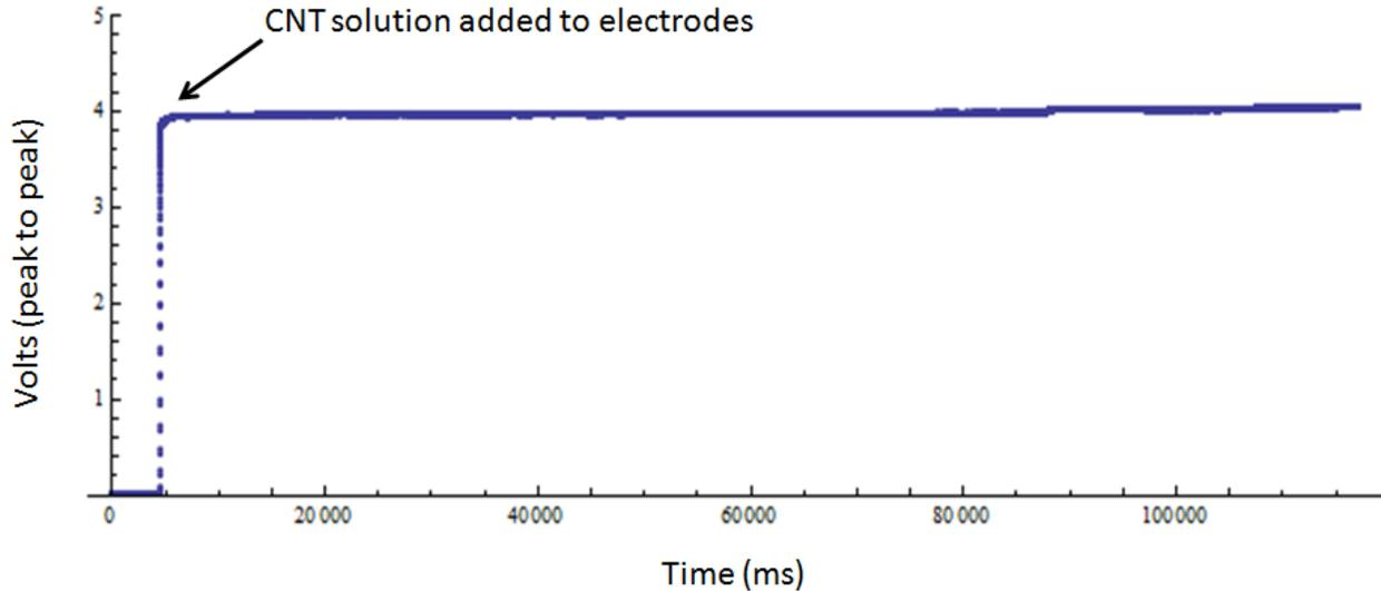
**Figure 4.6** Plot of measured voltage on the FEs during DEP. The voltage on the DEs was  $14 V_{pp}$ . Despite millisecond temporal resolution no voltage changes larger than a few mV were detected, though the lumped element analysis model predicted changes on the order of 500 mV.
