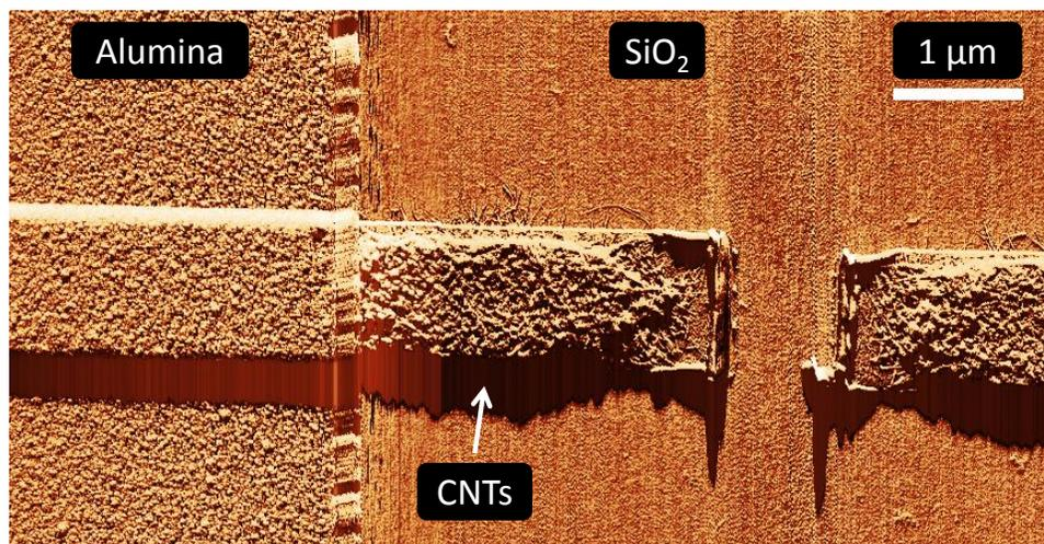
**Figure 3.9** Composite AFM amplitude image of region near the trap. A large portion of the region is covered in alumina (left). Bare areas of the FEs (which run left and right through the center of the image) can be seen in the immediate vicinity of the trap. A large mat of CNTs has been localized on all of the other parts of the FEs not covered in alumina.
