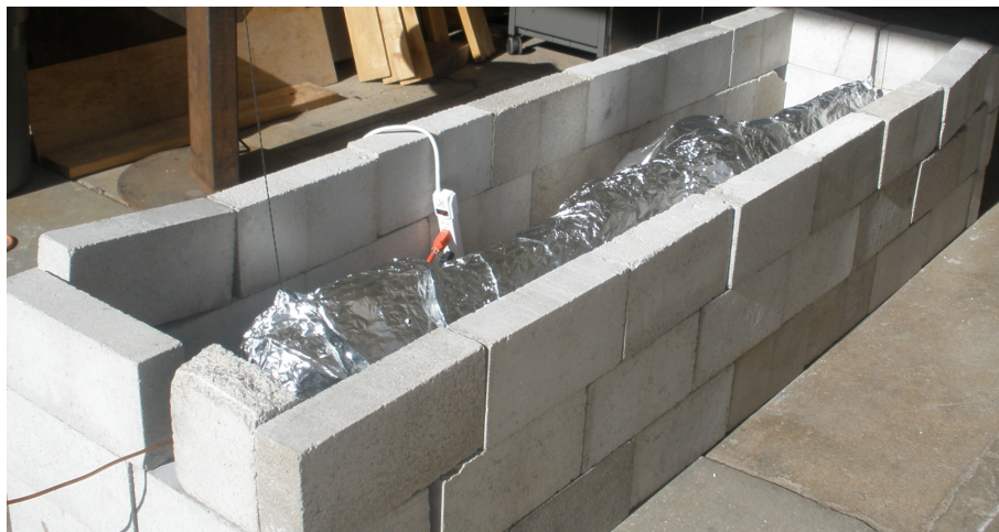
Figure E.1 Picture of the setup for baking out the interferometer chamber in air. After the chamber was wired with heat taped and wrapped in foil, crumpled aluminum foil was used to fill the remaining space in the cavity, and long sheets of foil were laid across the top. The chamber was baked at \sim 350^\circ\text{C} for 4 days.
