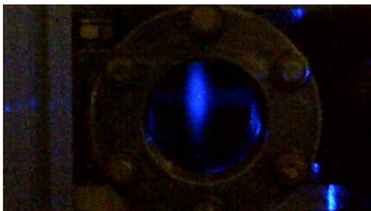
Figure 9.2 Picture of an ^{88}\text{Sr} MOT formed in the experiment. The bright dot in the middle of the fluorescence is the trapped atoms.
