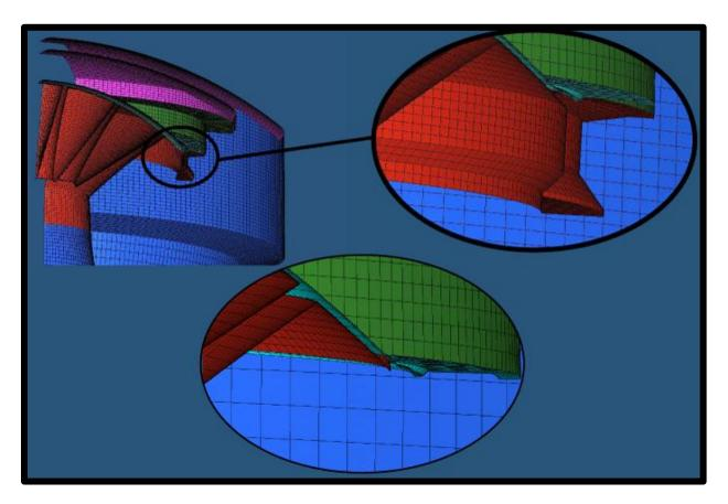
FIG. 5.12. Illustration of the gap in the BE mesh (top) that causes a parasitic resonance, and the reduced boundary (bottom) used to eliminate it.
