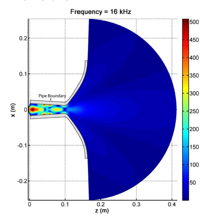
FIG. 4.17. Pressure magnitude of the interior pressure field for the  $120^{\circ}$  x  $60^{\circ}$  horn along the  $120^{\circ}$  cross section at 16 kHz.
