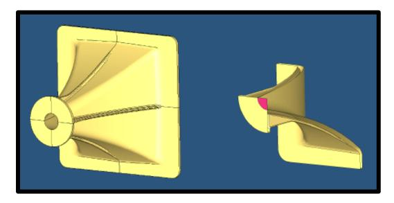
FIG. 4.1. Pictorial illustration of a full horn model and a reduced quarter of the model. Pink boundary represents excitation source.
