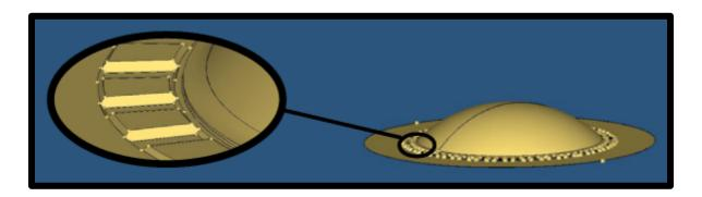
FIG. 5.2. Illustration of the compression driver diaphragm.
