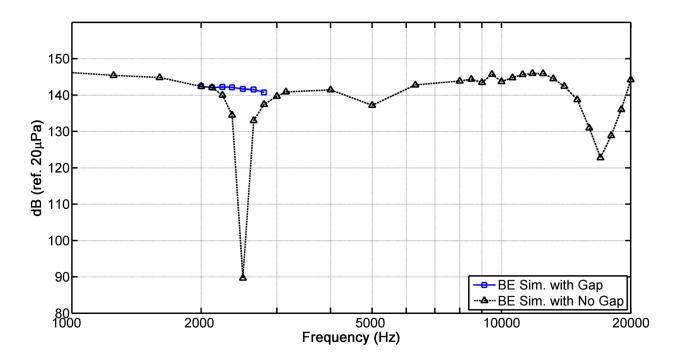
FIG. 5.13. Frequency response comparison at compression driver exit of an existing model with and without the boundary causing a parasitic resonance at 2.5 kHz.
