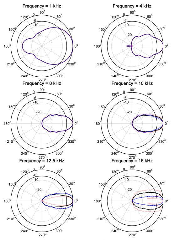
FIG. 4.8. Comparison of pressure directivity in dB (normalized to 0 dB) of a simulated  $30^{\circ}$  x  $45^{\circ}$  horn inward (---), outward (||||), and no curvature (—). The decibel value is indicated radially and 0 degrees is on-axis with the horn. The  $30^{\circ}$  slice is shown.
