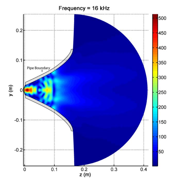
FIG. 4.20. Pressure magnitude of the interior pressure field for the  $120^{\circ}$  x  $60^{\circ}$  horn along the  $60^{\circ}$  cross section at 16 kHz.
