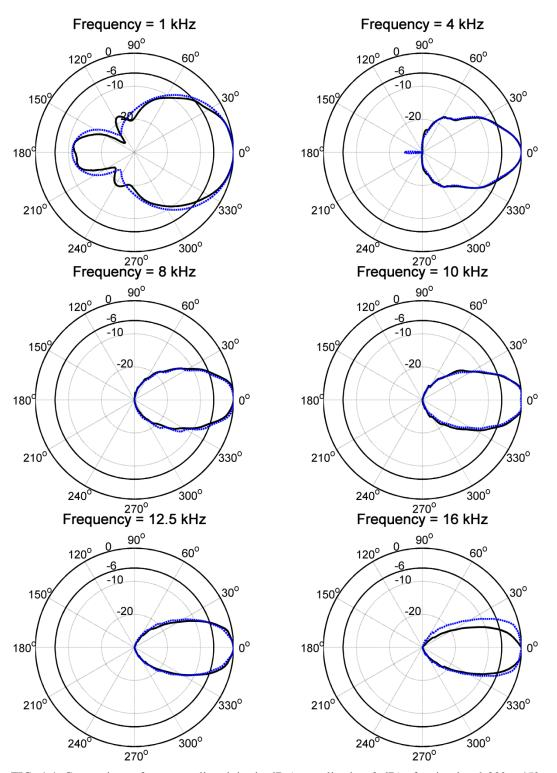
FIG. 4.4. Comparison of pressure directivity in dB (normalized to 0 dB) of a simulated  $30^{\circ}$  x  $45^{\circ}$  horn (---) and experimental measurement (—). The decibel value is indicated radially and 0 degrees is on-axis with the horn. The  $45^{\circ}$  slice is shown.
