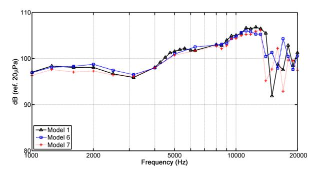
FIG. 5.15. Comparison of on-axis frequency response radiation for Model 1, 6, and 7.
