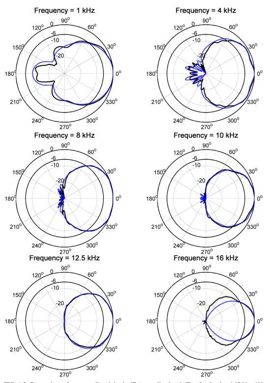
FIG. 4.5. Comparison of pressure directivity in dB (normalized to 0 dB) of a simulated  $120^{\circ} \times 60^{\circ}$  horn (---) and experimental measurement (—). The decibel value is indicated radially and 0 degrees is on-axis with the horn. The  $120^{\circ}$  slice is shown.
