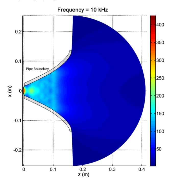
FIG. 4.19. Pressure magnitude of the interior pressure field for the  $120^{\circ}$  x  $60^{\circ}$  horn along the  $60^{\circ}$  cross section at 10 kHz.
