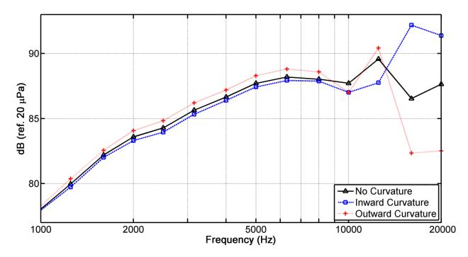
FIG. 4.12. Simulated results for on-axis frequency response of a 30° x 45° horn with different input wavefront curvatures.
