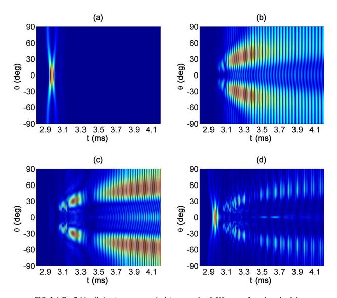
FIG. 3.6. Far-field radiation (pressure magnitude) measured at 0.508 meters from the exit of the pipe as a function of angle and time. (a) (0,0) mode. (b) (0,1) mode. (c) (0,2) mode. (d) Combination of several modes.
