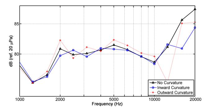
FIG. 4.13. On-axis frequency response numerical simulations of a  $120^{\circ}$  x  $60^{\circ}$  horn for different input wavefront curvatures.
