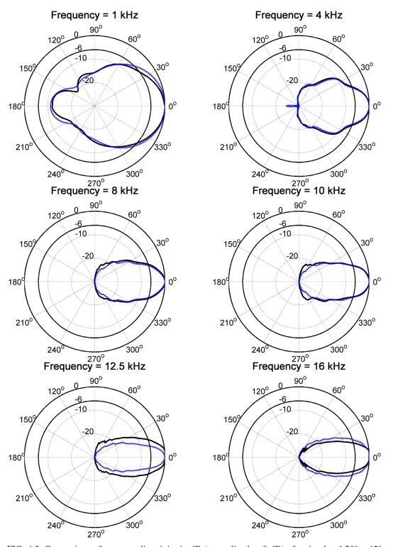
FIG. 4.3. Comparison of pressure directivity in dB (normalized to 0 dB) of a simulated  $30^{\circ}$  x  $45^{\circ}$  horn (---) and experimental measurement (—). The decibel value is indicated radially and 0 degrees is on-axis with the horn. The  $30^{\circ}$  slice is shown.
