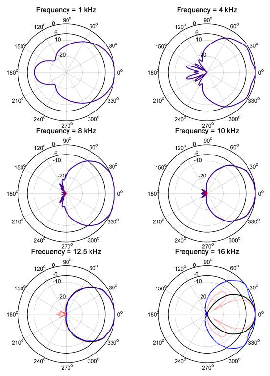
FIG. 4.10. Comparison of pressure directivity in dB (normalized to 0 dB) of a simulated  $120^{\circ}$  x  $60^{\circ}$  horn inward (---), outward (|||||), and no curvature (—). The decibel value is indicated radially and 0 degrees is on-axis with the horn. The  $120^{\circ}$  slice is shown.
