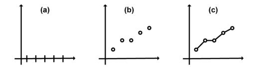
FIG. 2.2. (a) Chosen discrete x-values. (b) Output values of f(x) at discrete x-values. (c) Relationships between nodes (elements/lines connecting nodes).
