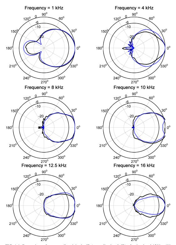
FIG. 4.6. Comparison of pressure directivity in dB (normalized to 0 dB) of a simulated  $120^{\circ} \times 60^{\circ}$  horn (---) and experimental measurement (—). The decibel value is indicated radially and 0 degrees is on-axis with the horn. The  $60^{\circ}$  slice is shown.
