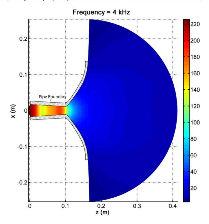
FIG. 4.15. Pressure magnitude of the interior pressure field for the  $120^{\circ}$  x  $60^{\circ}$  horn along the  $120^{\circ}$  cross section at 4 kHz.
