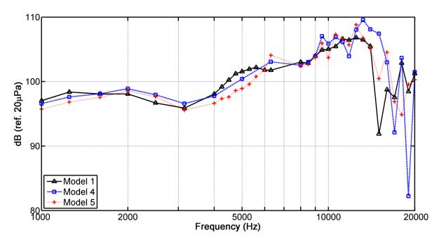
FIG. 5.15. Comparison of on-axis frequency response radiation for models 1, 4, and 5.
