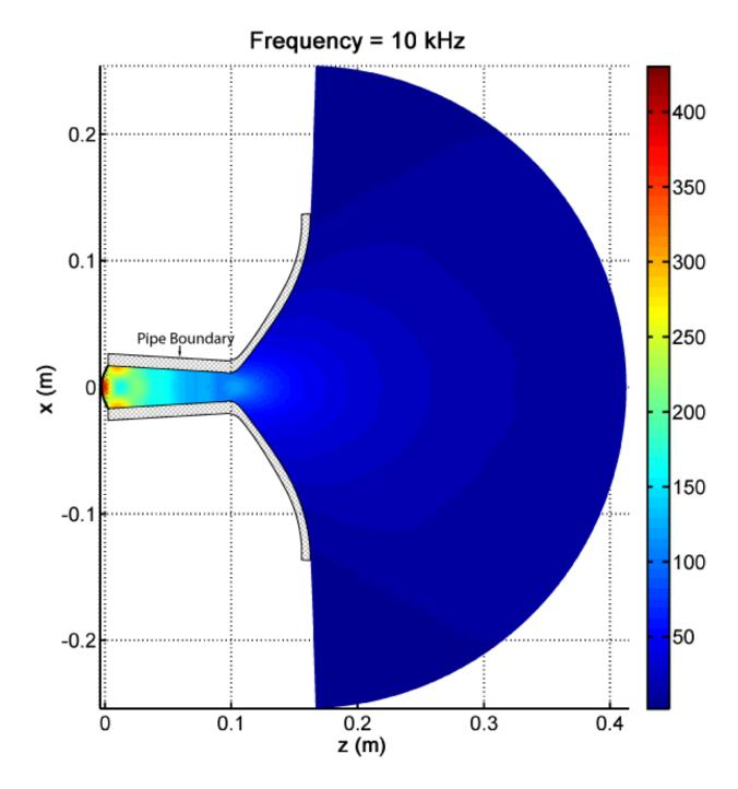
FIG. 4.16. Pressure magnitude of the interior pressure field for the  $120^{\circ}$  x  $60^{\circ}$  horn along the  $120^{\circ}$  cross section at 10 kHz.
