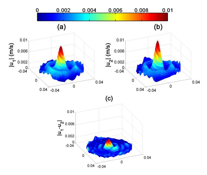
FIG. 5.5. (a) Scanning Laser Doppler Vibrometer (SLDV) measurement with no additional loading. (b) SLDV measurement with clay fit into outside edge of compression driver exit. (c) The magnitude of the difference of both velocity profiles.
