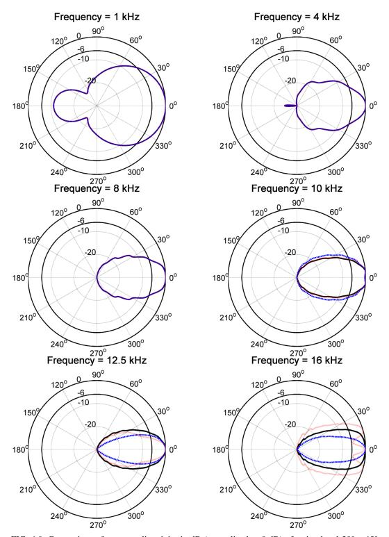
FIG. 4.9. Comparison of pressure directivity in dB (normalized to 0 dB) of a simulated  $30^{\circ}$  x  $45^{\circ}$  horn inward (---), outward (||||), and no curvature (—). The decibel value is indicated radially and 0 degrees is on-axis with the horn. The  $45^{\circ}$  slice is shown.
