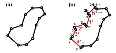
FIG. 2.3. (a) Geometry of a two-dimensional problem considered for Section 2.2.1.2. (b) Two-dimensional problem dissected into nodes and elements. Elements are indicated by the lines and starred (\*) numbers. Nodes are indicated by the circles and regular numbers.
