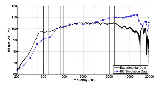
FIG. 5.10. Frequency response results for simulation and experiment of an ND6 compression driver on a  $45^{\circ}$  x  $30^{\circ}$  horn. Measurement is on-axis, 3.048 m from the entrance of the horn.
