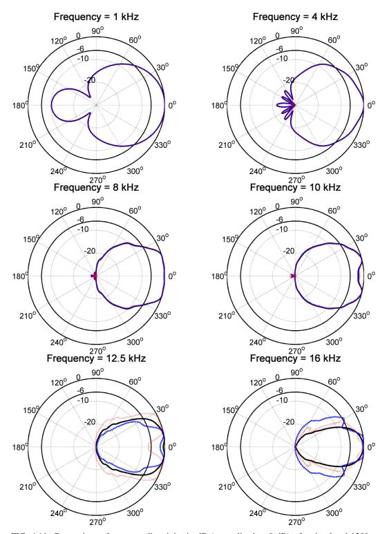
FIG. 4.11. Comparison of pressure directivity in dB (normalized to 0 dB) of a simulated  $120^{\circ}$  x  $60^{\circ}$  horn inward (---), outward (|||||), and no curvature (—). The decibel value is indicated radially and 0 degrees is on-axis with the horn. The  $60^{\circ}$  slice is shown.
