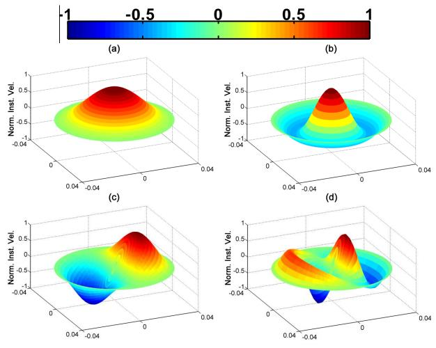
FIG. 5.3. Predicted modes for a spherical cap. Mode: (a) (0,0); (b) (0,1); (c) (1,0); (d) (1,1).
