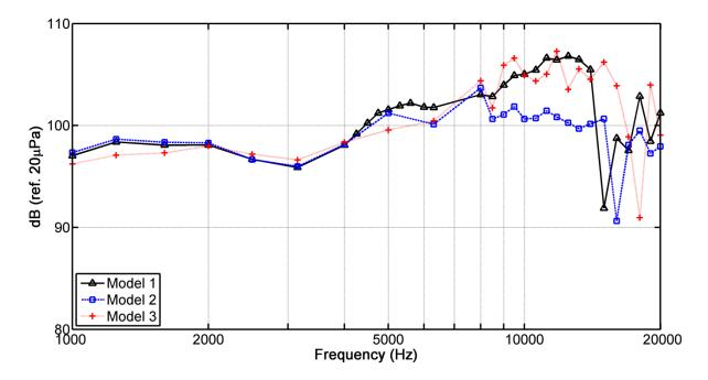
FIG. 5.14. Comparison of on-axis frequency response radiation for models 1, 2, and 3.
