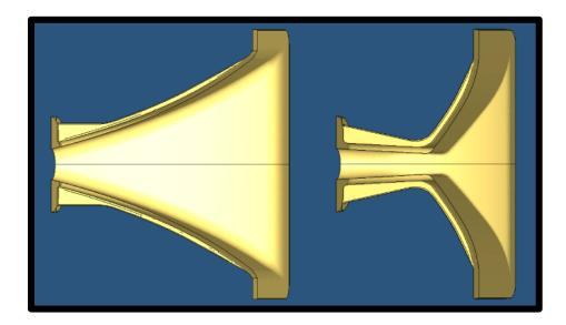
FIG. 4.14. Side view of the horns simulated in Sec. 4.3. The  $30^{\circ}$  cross section of the  $30^{\circ}$  x  $45^{\circ}$  horn is shown on the left and the  $120^{\circ}$  cross section of the  $120^{\circ}$  x  $60^{\circ}$  horn is shown on the right.
