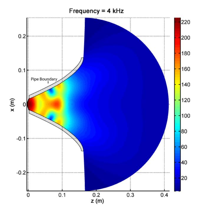
FIG. 4.18. Pressure magnitude of the interior pressure field for the  $120^{\circ}$  x  $60^{\circ}$  horn along the  $60^{\circ}$  cross section at 4 kHz.
