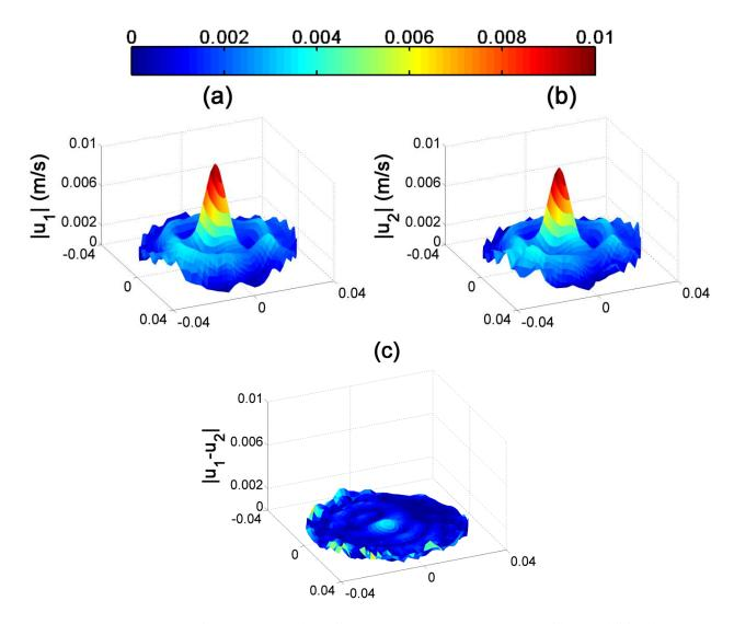
FIG. 5.6. (a) Scanning Laser Doppler Vibrometer (SLDV) measurement with no additional loading. (b) SLDV measurement with a  $30^{\circ}$  x  $45^{\circ}$  horn mounted to the compression driver. (c) The magnitude of the difference of both velocity profiles.
