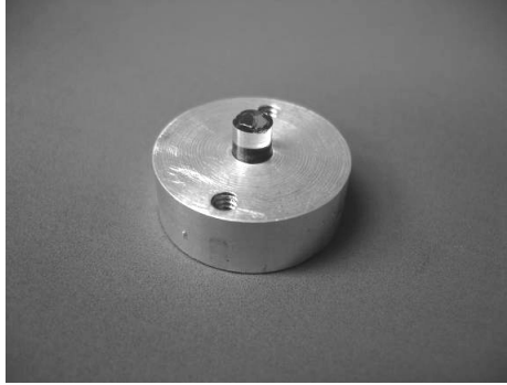
Figure 2.5 Completed aluminum cylinder with glass rod sample holder cemented in place.
