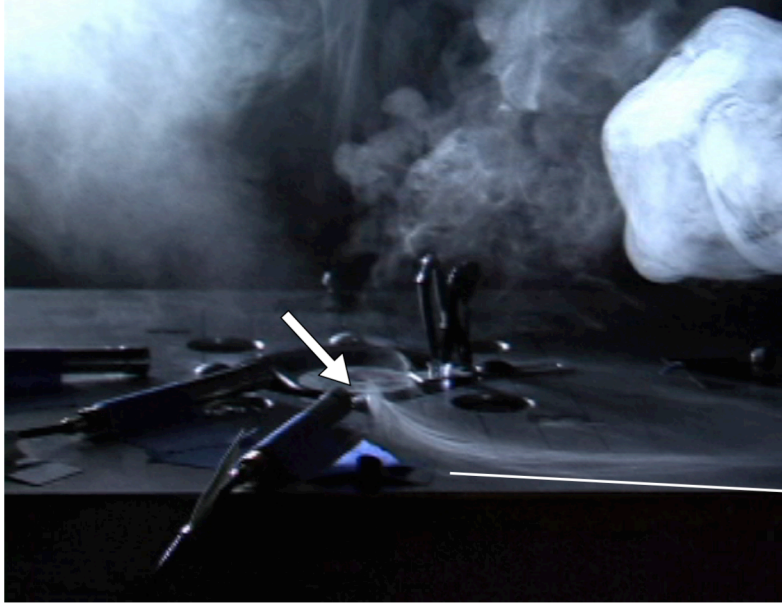
Figure 6.5 Flow visualization of DC-powered fan in arrangement 1 with fog machine outside of enclosure
