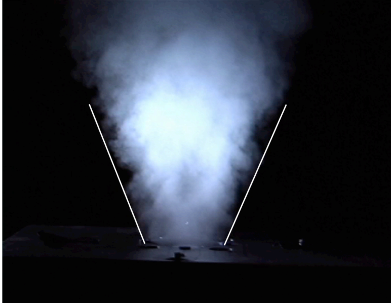
Figure 6.6 Flow visualization of PWM-powered fan in arrangement 1
