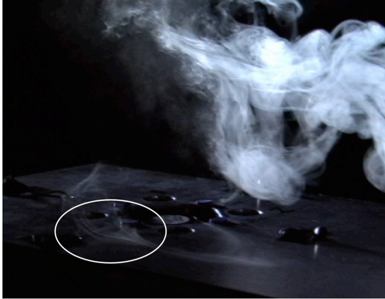
Figure 6.8 Flow visualization of PWM-powered fan in arrangement 3 with fog machine outside of enclosure
