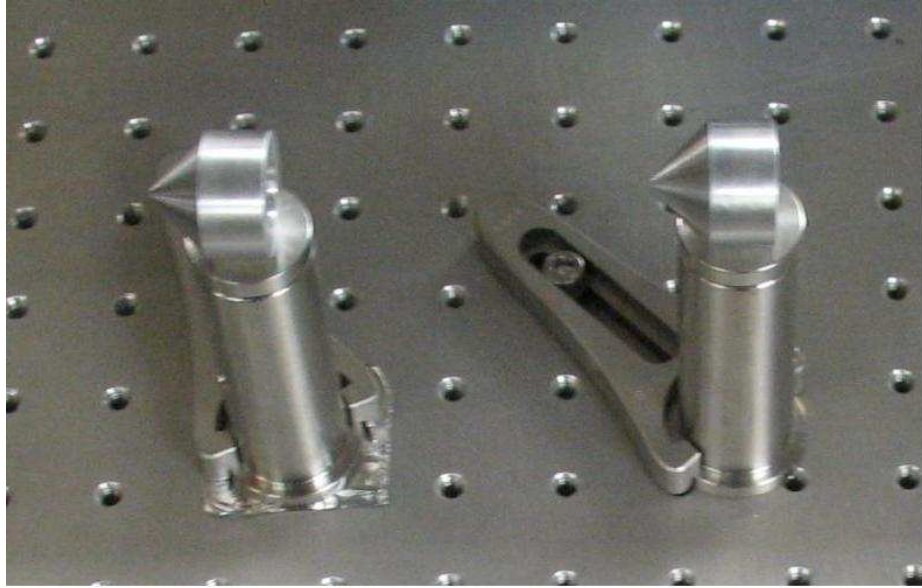
Figure 4.2 Skimmers used to define the direction and divergence of the atom beam.
