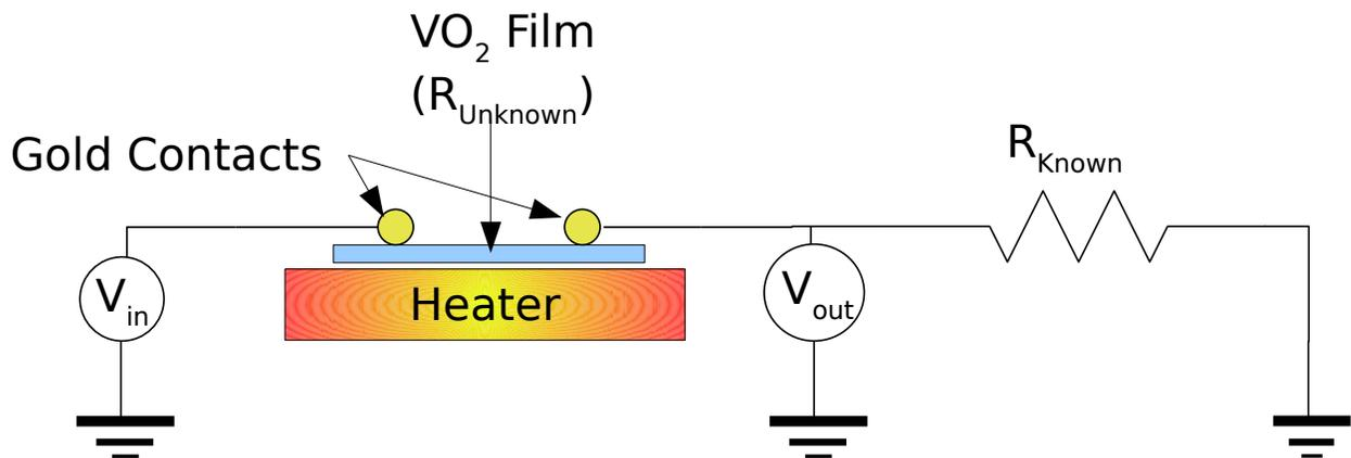
**Figure C.5** Diagram showing how the film resistance was measured during the transition. A voltage divider circuit was set up with a reference resistance. The contacts to the film were gold balls mechanically in contact with the film.
