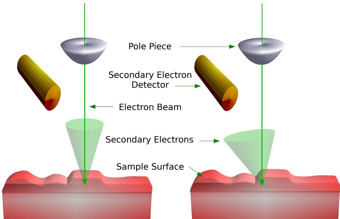
**Figure 1.7** Using the Secondary Electron Detector in the Scanning Electron Microscope, contrast is obtained by the number of secondary electrons detected. The number of secondary electrons that “leave” the surface of the sample depends on the the angle between the main beam and the surface
