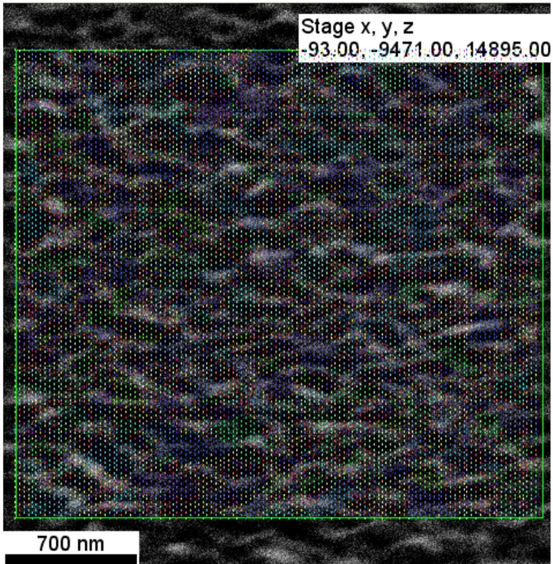
**Figure 1.13** (color) During an OIM scan two important factors to consider are the grain size, and the scan size. In this sample image, the grain size is approximately 300 nm across and the distance between sampling points is about 50nm.
