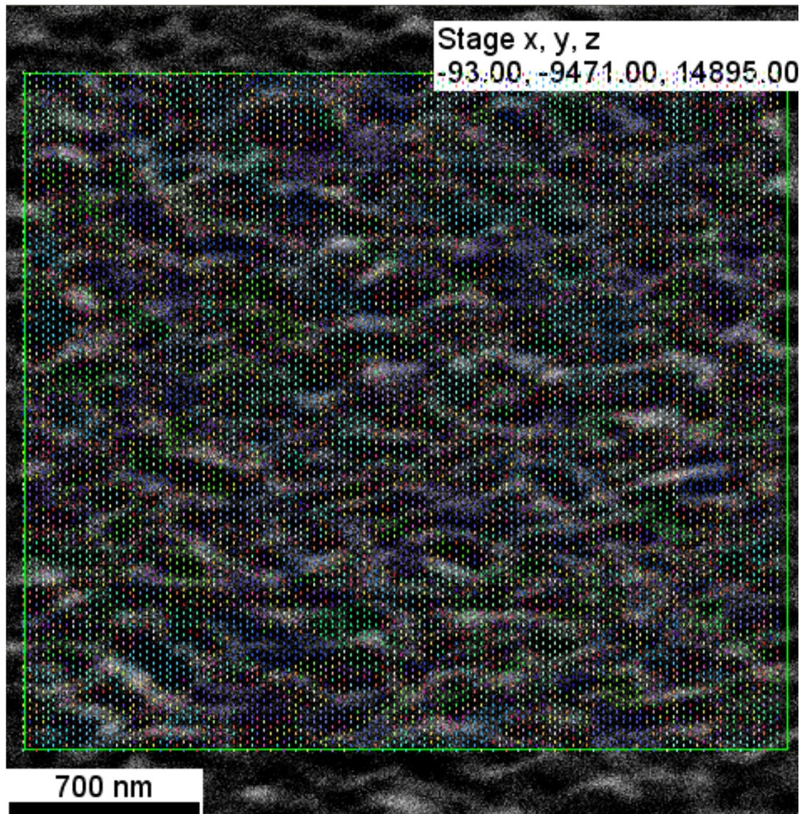
**Figure 2.11** [Color] In the Background, an SEM image is used as a reference. Recall that the sample is tilted  $70^\circ$ . An area is selected to perform an OIM scan, the separation between samples is specified, and the type of grid chosen. In this case, an area approximately  $3\mu\text{m}$  (along the x direction) is probed every 50 nm using a hexagonal grid.
