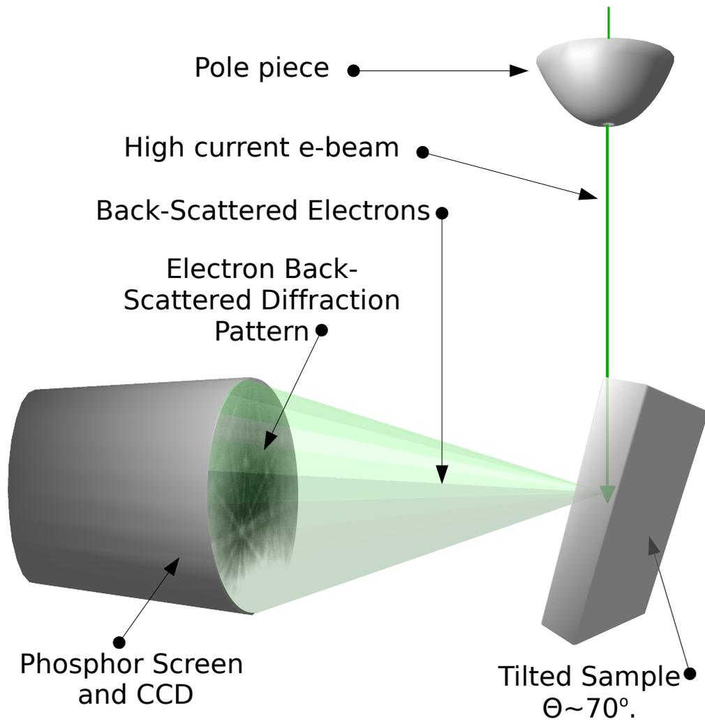
**Figure 1.11** As the electron beam interacts with the sample, some of the electrons will be “back-scattered” in the Bragg Condition. These electrons will form Kikuchi patterns that can be detected with a phosphor screen and a camera. In Orientation Imaging Microscopy, Kikuchi patterns are recorded and indexed as a scan takes place in the Scanning Electron Microscope.
