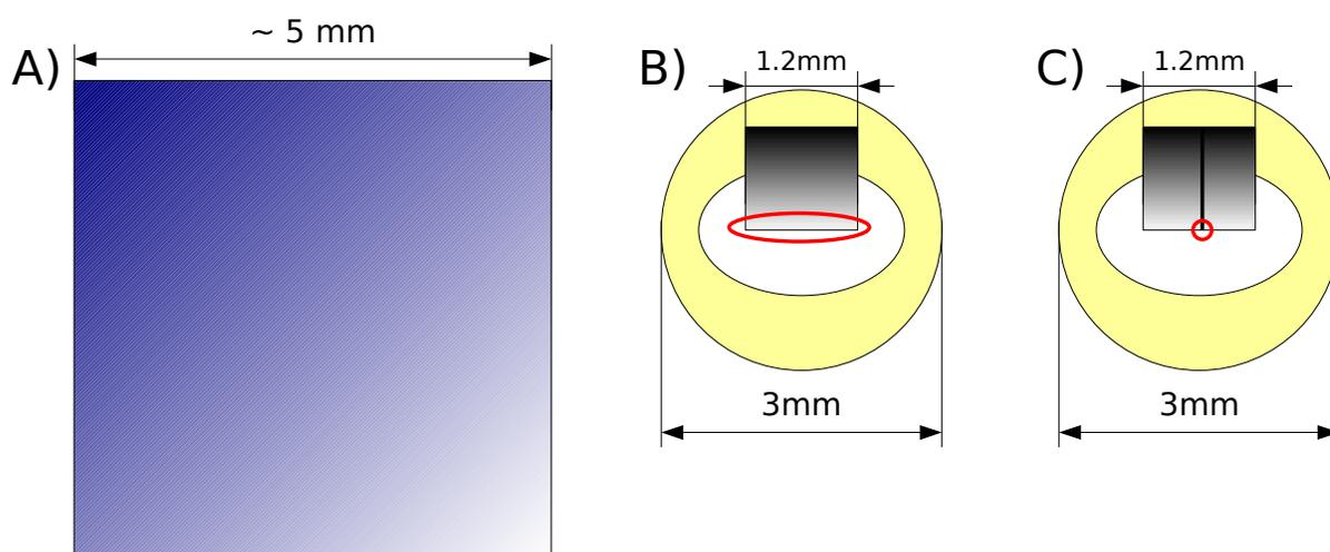
**Figure C.3** Size comparison between A) a typical SEM sample used, and two TEM samples, B) a plan-view and C) a cross-sectional view. While the SEM can image the whole surface, the imageable area is greatly reduced in the TEM samples.
