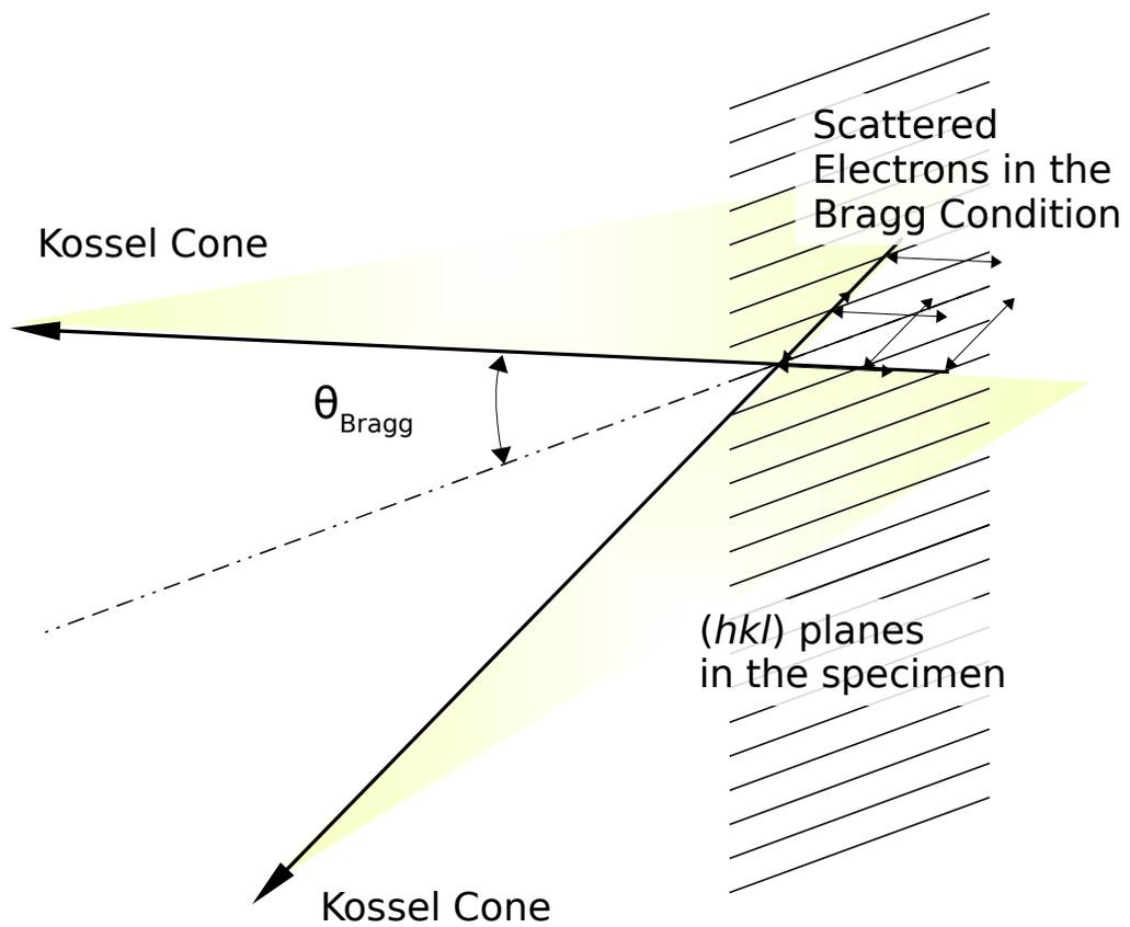
**Figure 1.9** Since the electrons from the main beam scatter in all directions, a number of them will find themselves in the Bragg condition. Kossel cones are created from all the electrons scattering in the Bragg condition.
