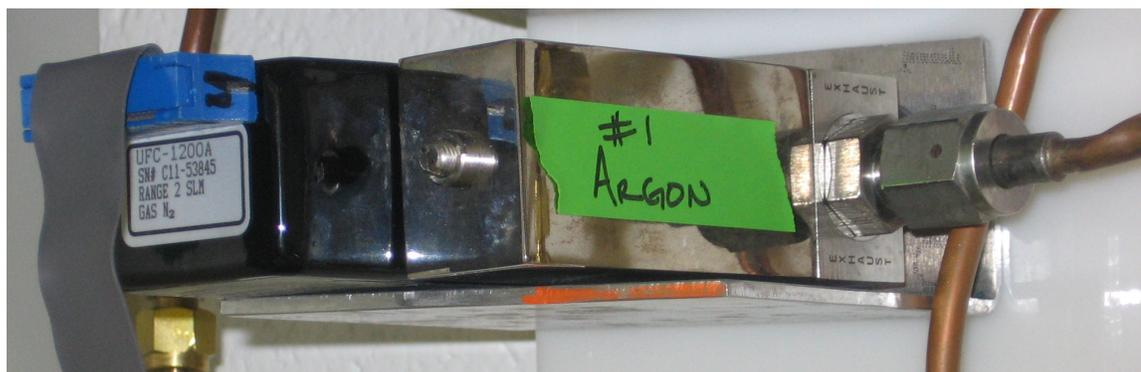
**Figure 2.6** Mass Flow Controller used to control the argon flow.
