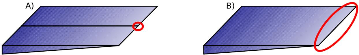
**Figure C.2** TEM “wedge” samples for A) a cross-sectional view, where the film is “sandwiched” between two silicon pieces in order to view its thickness; and B) a plan-view where the substrate is polished thin leaving the film undisturbed along the edge
