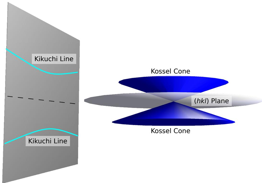
**Figure 1.10** Kikuchi lines are the intersections of Kossel cones with the phosphor screen. (The bands are actually hyperbolic not parallel. However, due to the small angle between the plane and the cone, they look like parallel lines in practice.)
