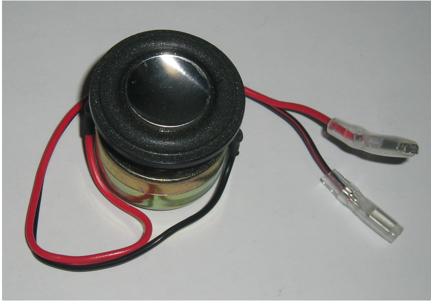
Figure 5-6: A photograph of the 25-mm loudspeaker that was used as a control actuator in the ANC system.
