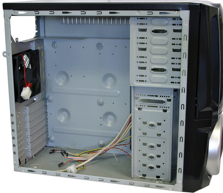
Figure 1-1: A common axial cooling fan installation (left side of the machine) inside a computer case 1 .
