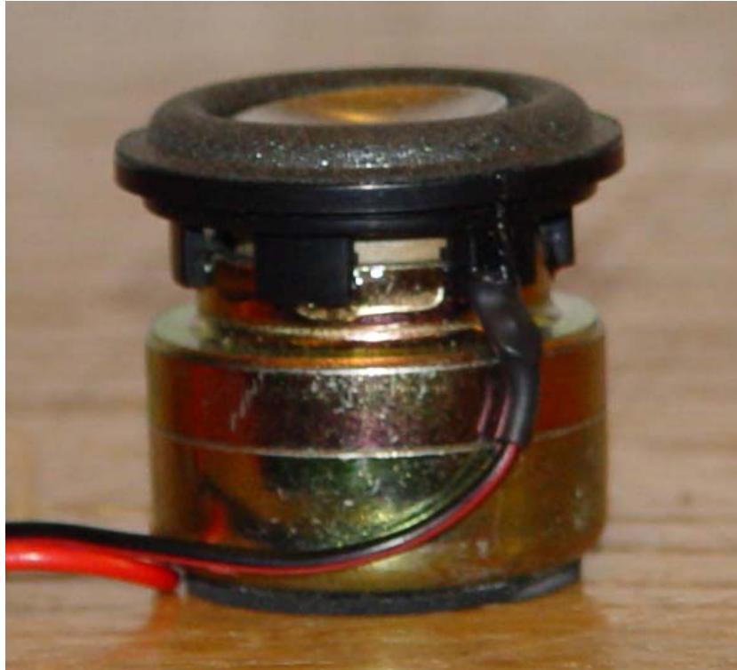
Figure 4.2 1” Loudspeaker used as secondary source for ANC.
