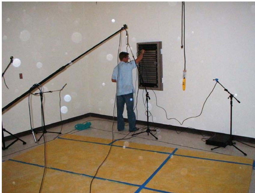
FIG. 2.3. Test material placed in Type A mounting.
