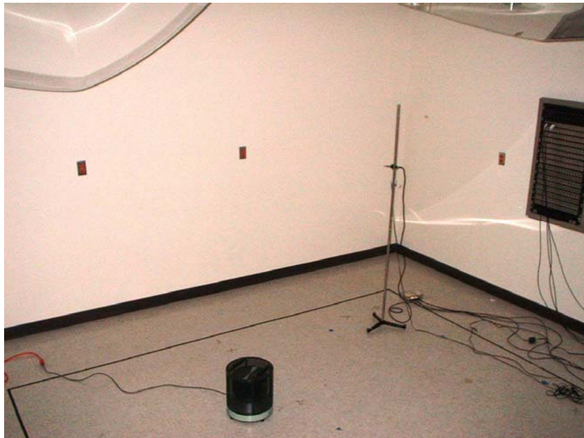
FIG. 2.9. Placement of sound source in a reverberation chamber.
