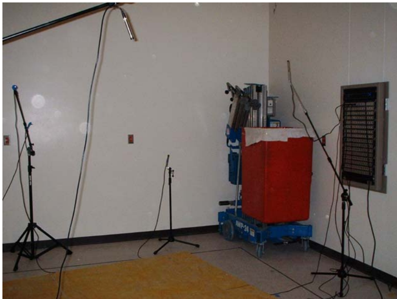
FIG. 2.2. Genie Lift™ positioned as a diffuser during room qualification.
