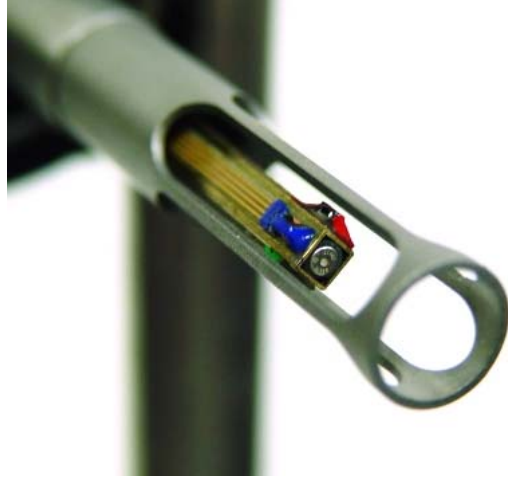
FIG. 2.11. Detailed view of Microflow™ sensor.
