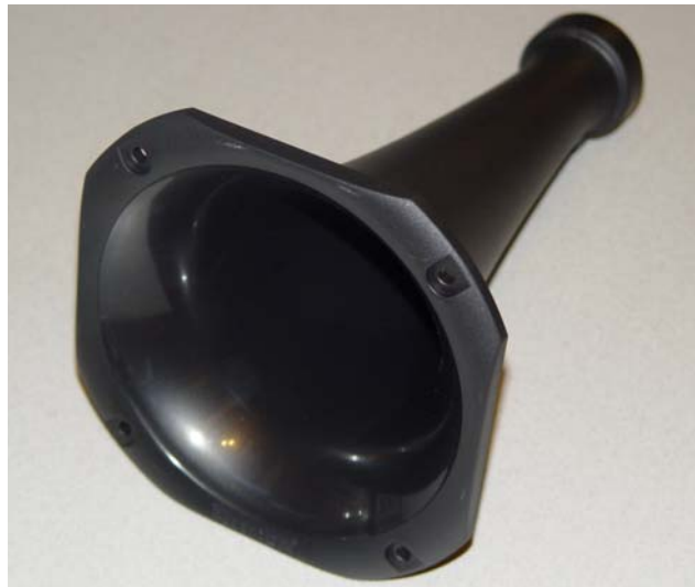
Figure 8.17. High-frequency horn attached to the compression driver. A Selenium HL14-25 exponential horn.
