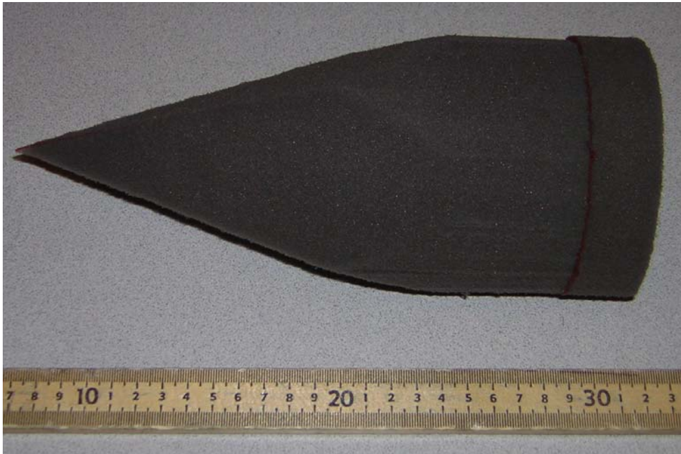
Figure 6.2. Foam wedge placed in the end of the tubes to give an anechoic termination. The ruler at the bottom of the figure is marked in centimeters.
