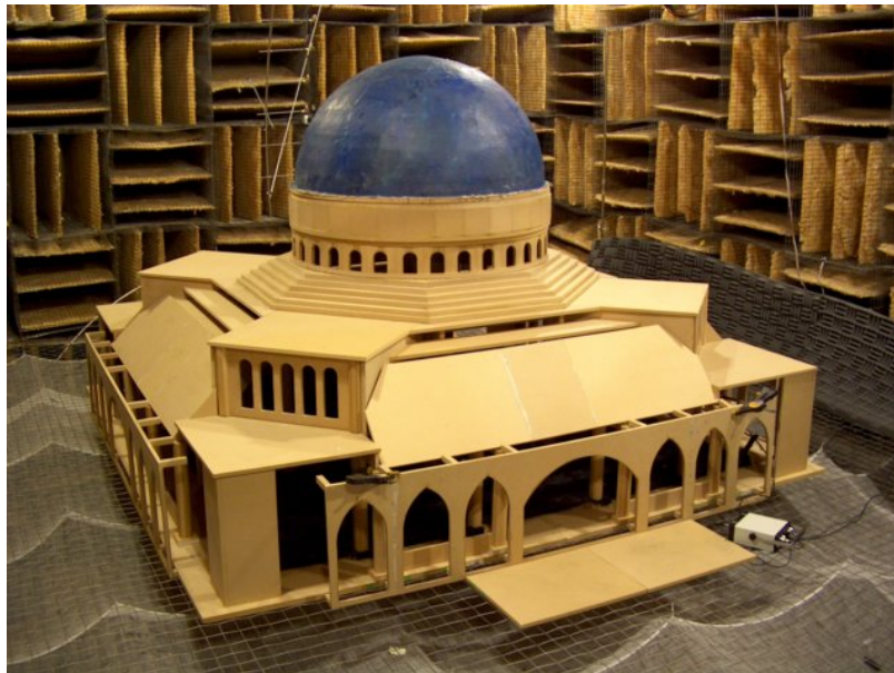
Figure 5.1. The scale model in the BYU anechoic chamber.
