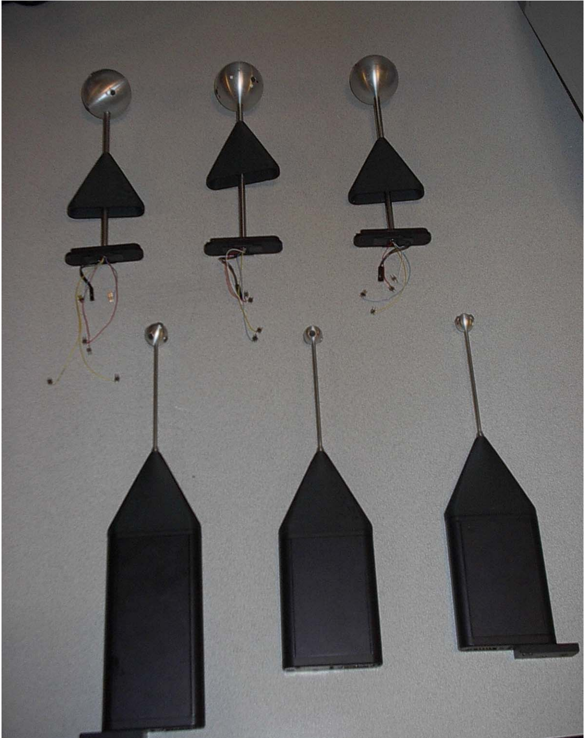
Figure 3.2: Large Six Microphone Probe, Large Tetrahedron Probe, Large Orthogonal Probe, Small Six Microphone Probe, Small Tetrahedron Probe, Small Orthogonal Probe
