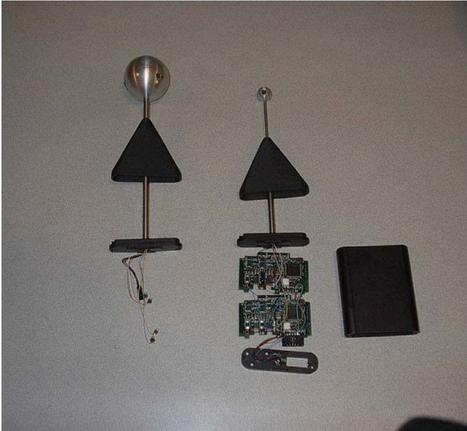
Figure 3.1: Large and Small Tetrahedron Probe, 2 DSITs, and Aluminum Case
