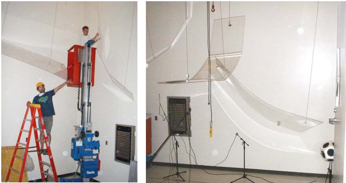
Figure 6.1. Diffusers being hung to satisfy the ISO 354 qualification procedure for reverberation chamber measurements.
