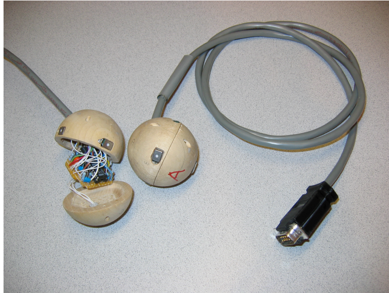
Figure 2.1 3D ED sensors. The left sensor is open to reveal the electronics.
