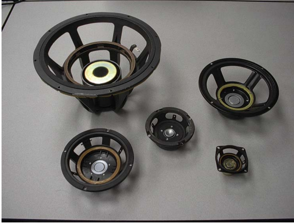
Fig. 2.7. Photograph of driver frames and magnet structures remaining after the destructive evaluation technique.
