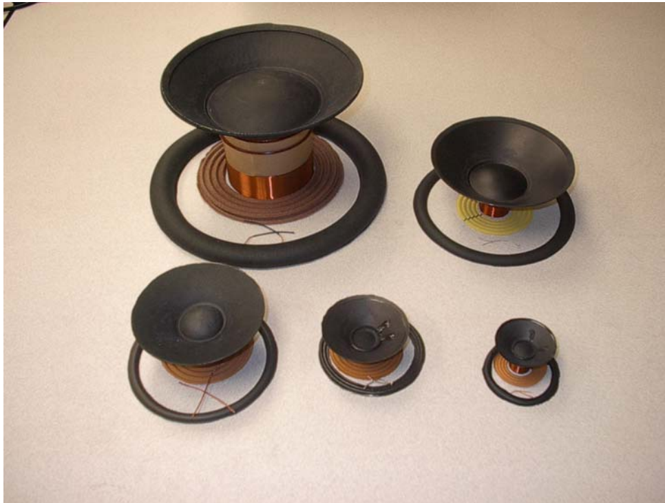
Fig. 2.6. Photograph of cone assemblies and suspension system pieces of drivers used in the destructive evaluation technique for M_{MD} .
