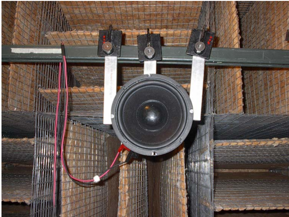
Fig. 4.3. Photograph of a driver in a free-field configuration with its axis horizontal.
