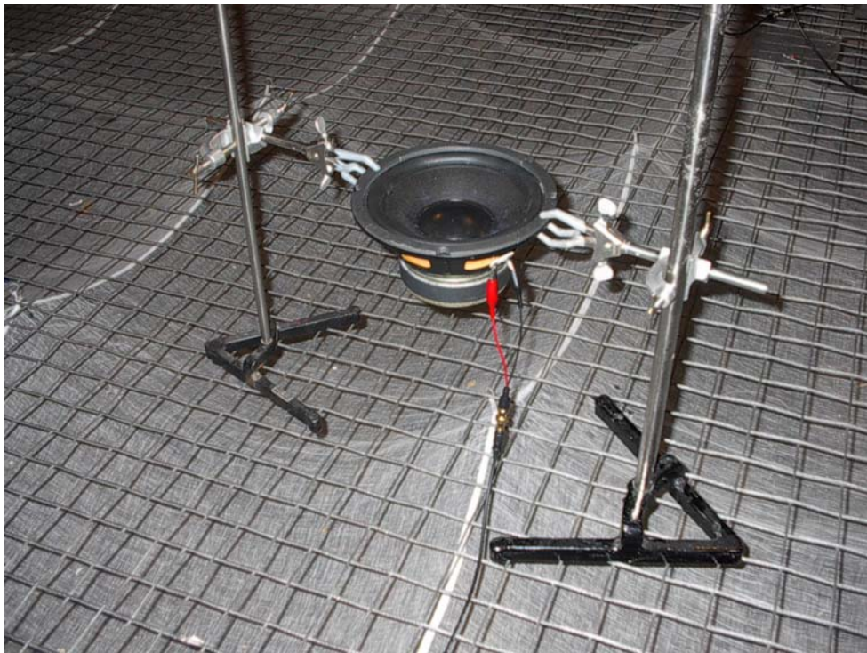
Fig 4.1. Photograph of a driver in a free-field condition with its axis vertical.
