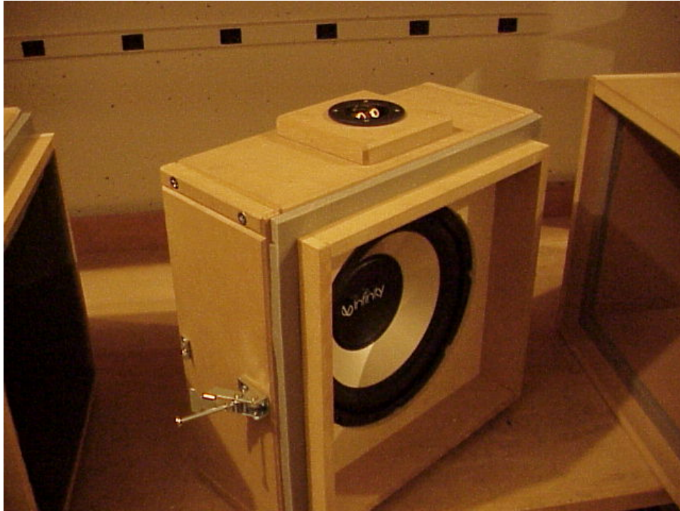
Fig. 5.6. Photograph of the partition containing mounted driver number 2 in a surrounding baffle.
