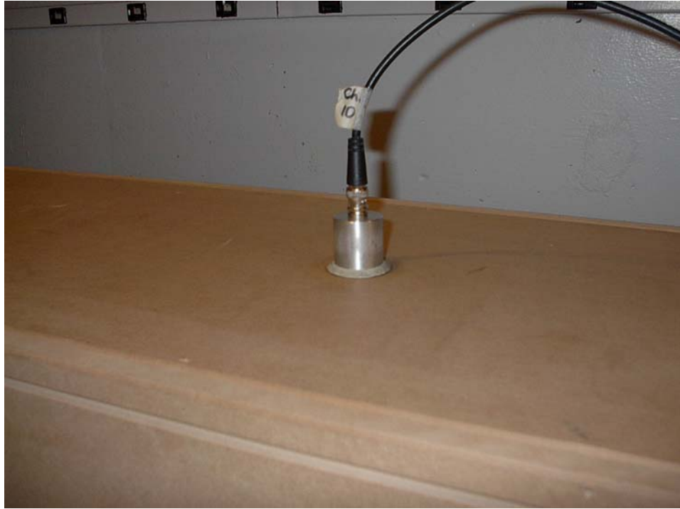
Fig. 5.8. Photograph of a microphone used in the plane wave tube measurements (outside view).
