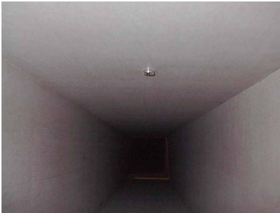
Fig. 5.9. Photograph of a microphone used in the plane wave tube measurements (inside view).
