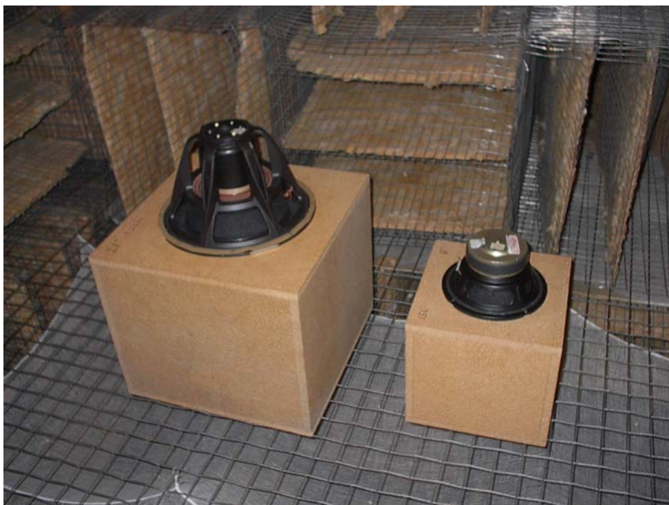
Fig. 4.5. Photograph of two sample drivers placed on test boxes with their axes vertical.
