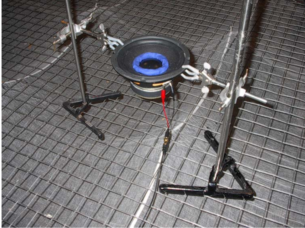
Fig. 4.2. Photograph of a driver in an added-mass configuration with its axis vertical.
