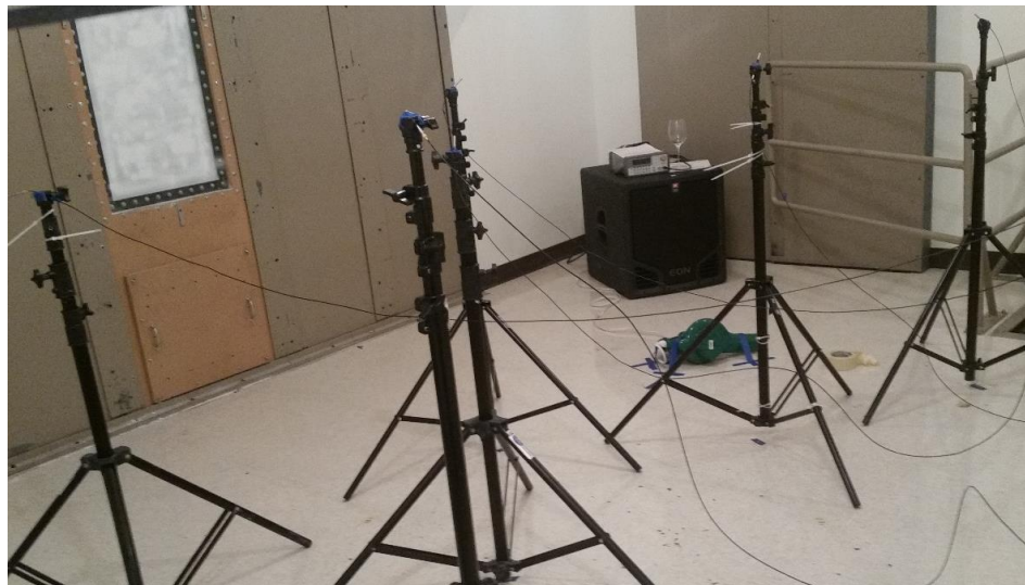
Figure 2. Reverberation chamber measurement of the leaf blower with six microphones.
