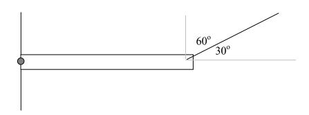
Problem 24. A 3 meter long uniform beam of unknown weight is attached to a wall and supported by a cable that provides a force upward and to the right. It attaches at the right end of the beam. The force the cable supplies is 5500 N. This causes a torque of [24?]
