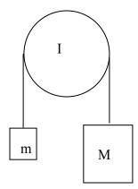
29. Looking at the forces on the pulley: if the tension from  $M(T_M)$  were not larger than the tension from  $m(T_m)$ , the pulley would not start rotating clockwise (as it obviously must.) So there must be a net torque. Choice b
